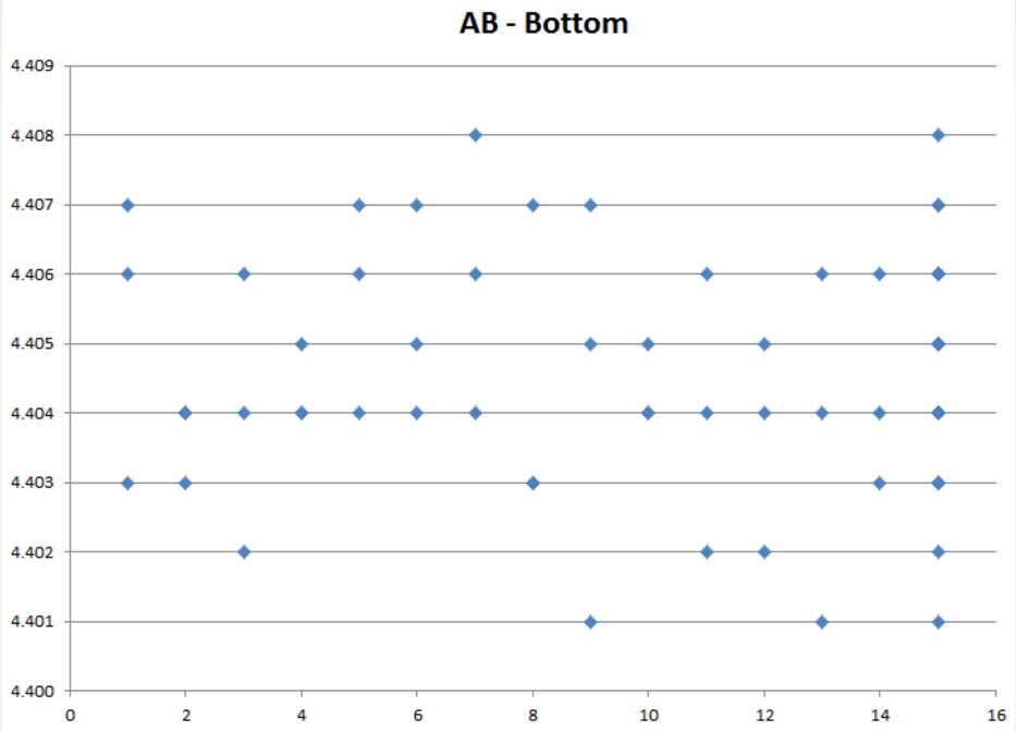
Notice that the Distance AB, measured at the Bottom of the part, varies from 4.401" to 4.408" (a range of 0.007"). This range of variation at the closed end is much tighter than at the open end. The steel dimension is 4.416". This implies that the shrink factor ranges from 0.002 - 0.003 in/in . The shrink factor applied in the tool was 0.002 in/in for BMC 605. The measured shrinkage for AB at the Bottom is in line or just a little higher than the recommended shrinkage for BMC 605.
