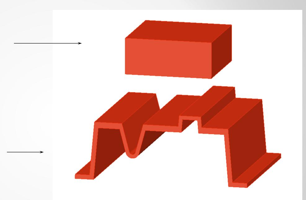
We then performed a Thermoset Compression Molding simulation with Moldflow Scandium. The solid model of the part and external initial charge were pulled into Moldflow Scandium.
