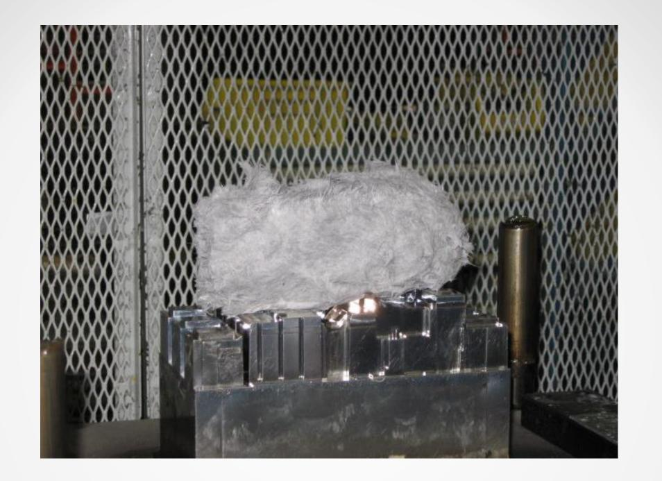
This picture shows how a charge of Thermoset BMC is typically placed on top of the B-Half of the mold prior to compression.
