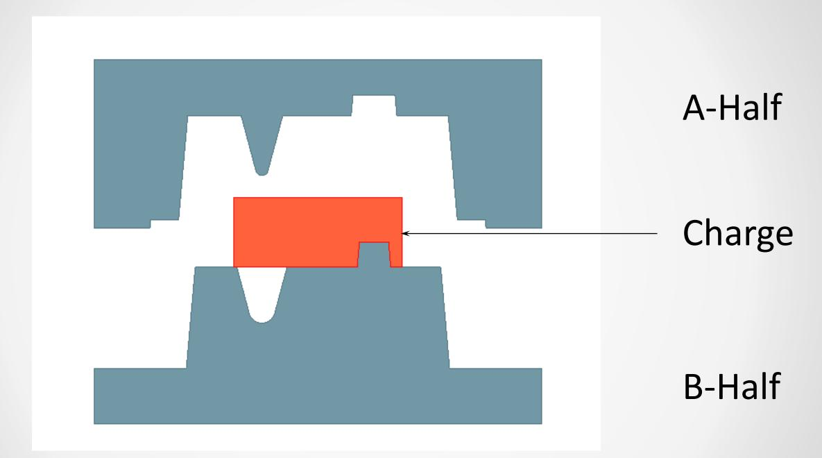
We first show a graphical depiction of an actual compression molding process where a Thermoset BMC charge is compressed between two die halves.
