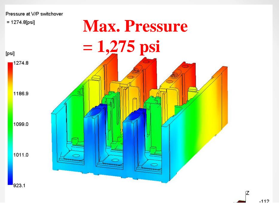
With BMC 605, results of our analysis showed that the Compression Pressure required to fill the part would be 1,275 psi. Shown on the next Slide is the actual hydraulic pressure measured off a dial gauge at the press.
