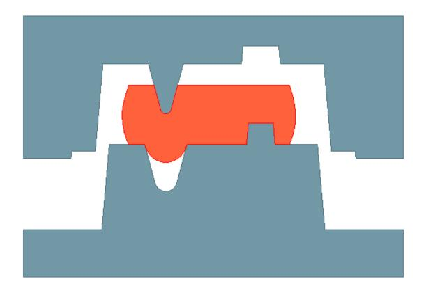
As the A-half moves down, the charge is further deformed. Notice that other than the protrusion on the upper die, the rest of the tool has not made contact with the charge.
