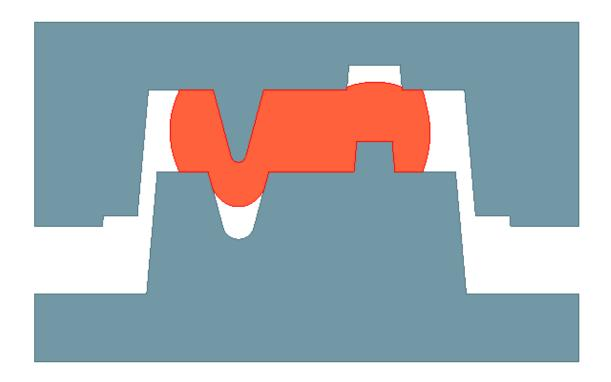
At this stage of movement of the A-half, notice that the entire upper surface of the charge comes into contact with the die. Material starts to bulge into the cut-out in the upper surface of the cavity.
