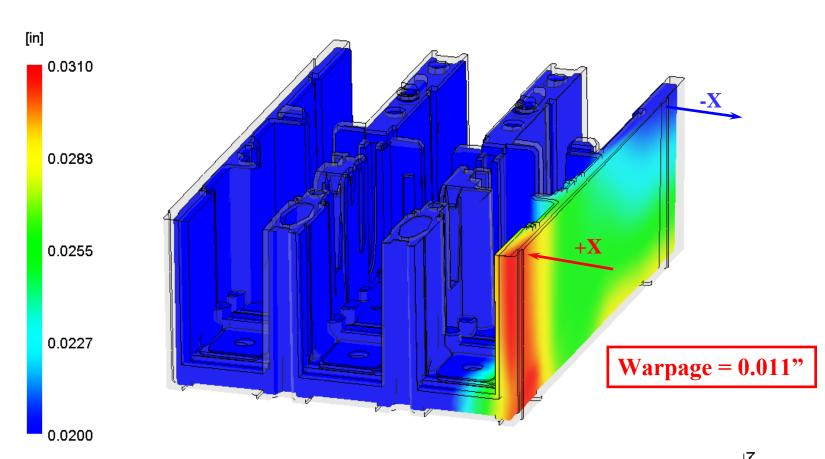
Warpage predicted was roughly 0.011" in the X-direction at the top of one of the side walls. Actual warpage measured in the molded parts was roughly 0.017". Therefore, the predicted warpage is roughly 35% lower than the measured warpage. These predictions are on the same order of magnitude of what was measured and is quite good considering all the variables that influence shrinkage and warpage.
