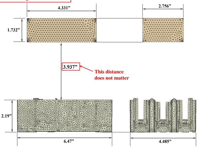
Q2R, 3Pole Base, Model/Mesh: Part & Charge Placement
