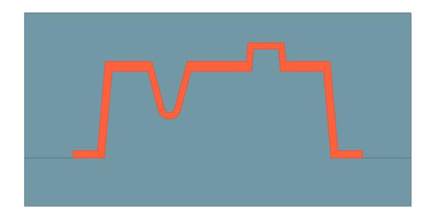
End of compression. A-half shuts off on B-half at the Parting Line. Notice that only at this stage, the wall thicknesses have the dimensions of the final part.
