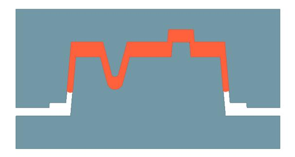
At this stage of compression, the lower surface of the A-half and the upper surface of the B-half are completely in contact with the charge and the polymer has moved down significantly to form the side walls. Notice the thickness of the side walls are larger than the final part side wall thickness.
