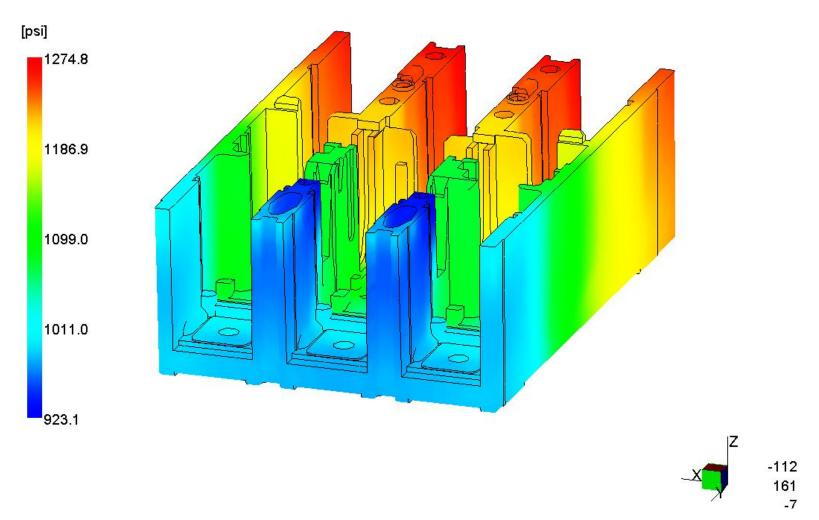
With BMC 605, results of our analysis showed that the Compression Pressure required to fill the part would be 1,275 psi. Shown on the next Slide is the actual hydraulic pressure measured off a dial gauge at the press.
