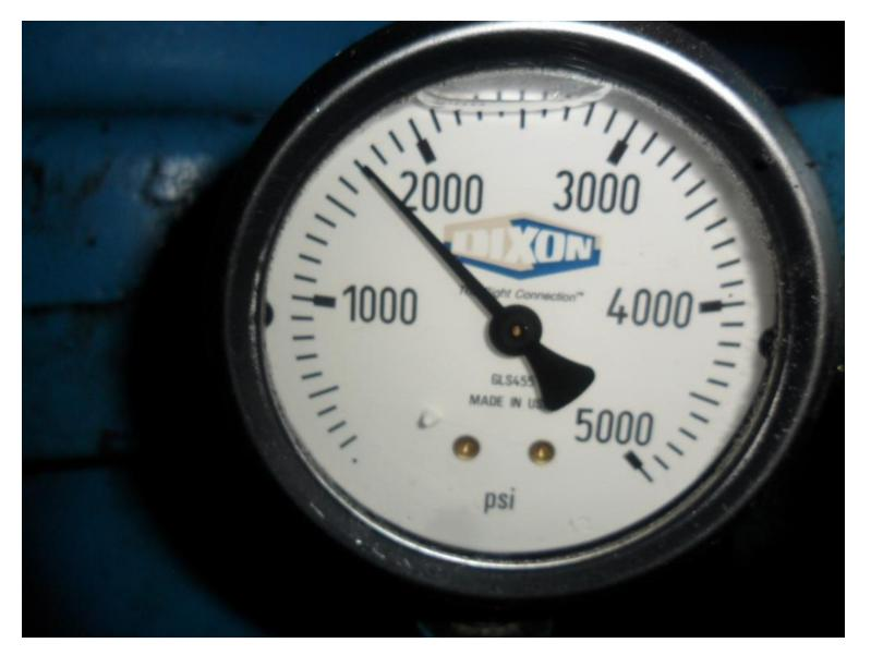
Pressure Gauge on the machine showed roughly 1,700 psi Hydraulic Pressure during the cure cycle. However, we do not have sufficient information from the molder as to how this pressure translates to Compression Force on the platen of the mold.
