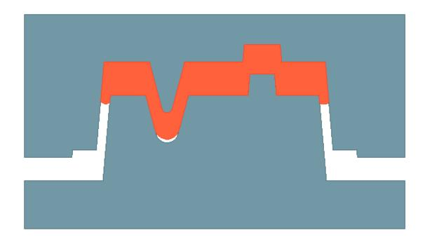
As the A-half moves down further, the upper surface of the charge has completely contacted the upper die. The U-shaped cut-out on the lower die is almost filled, while the polymer has started to move down the edges of the B-half to form the side walls.
