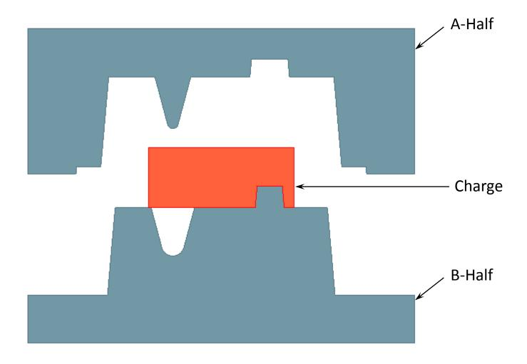
We first show a graphical depiction of an actual compression molding process where a Thermoset BMC charge is compressed between two die halves.
