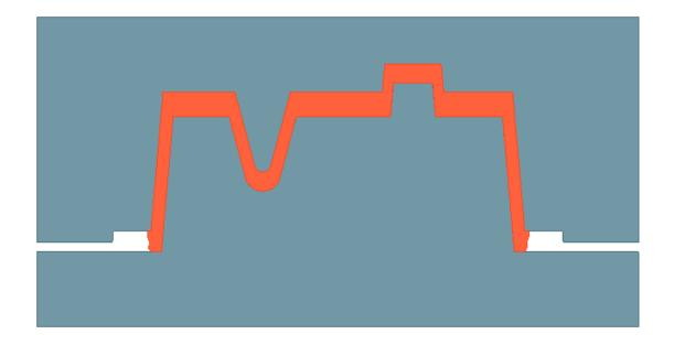
The polymer has now been squeezed all the way to the parting line. The only portion of the cavity yet unfilled are the flanges on the bottom.
