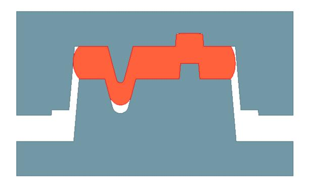
At this stage of compression, notice that the charge has come into contact with most of the upper surface of the cavity. However, it has not completely filled the U-shaped cut-out on the B-half.
