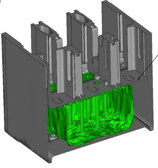
Upper Surface of the part is stretched in the Z direction to represent the upper die
