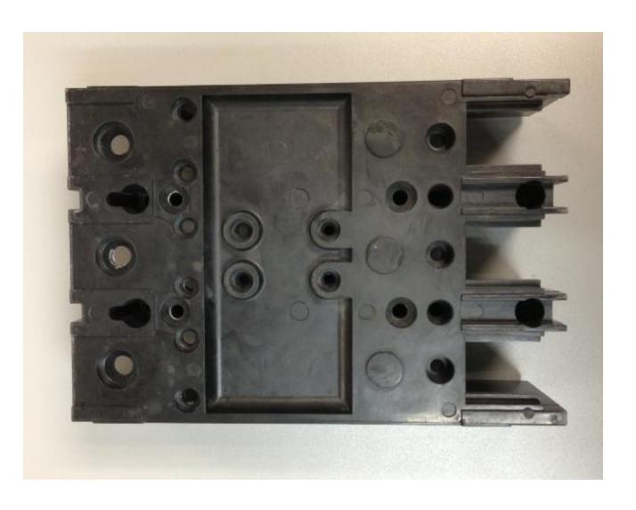
Q2R, 3Pole Base, Compression Molding Model/Mesh: Part & Charge Placement
