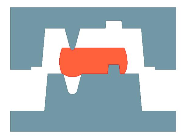
As the A-half starts to move down the upper surface of the charge is penetrated by any protrusion that may exist on the upper die. This displaces some of the volume and the charge starts to deform.
