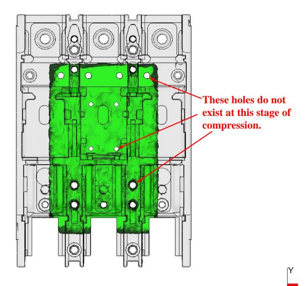
To avoid the holes at the start of compression, a thin web needs to modeled over each of the holes (thickness: 0.010" – 0.020")
