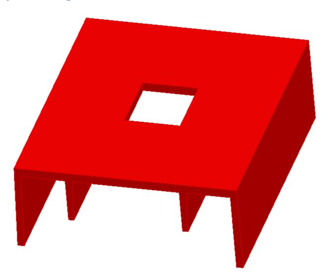
In order to simulate the model with a hole, we need to model the hole as a thin area (with thickness of around 0.010" – 0.020").
