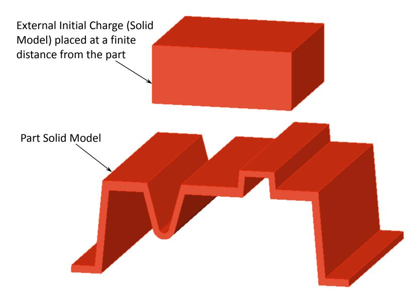
We then performed a Thermoset Compression Molding simulation with Moldflow Scandium. The solid model of the part and external initial charge were pulled into Moldflow Scandium.
