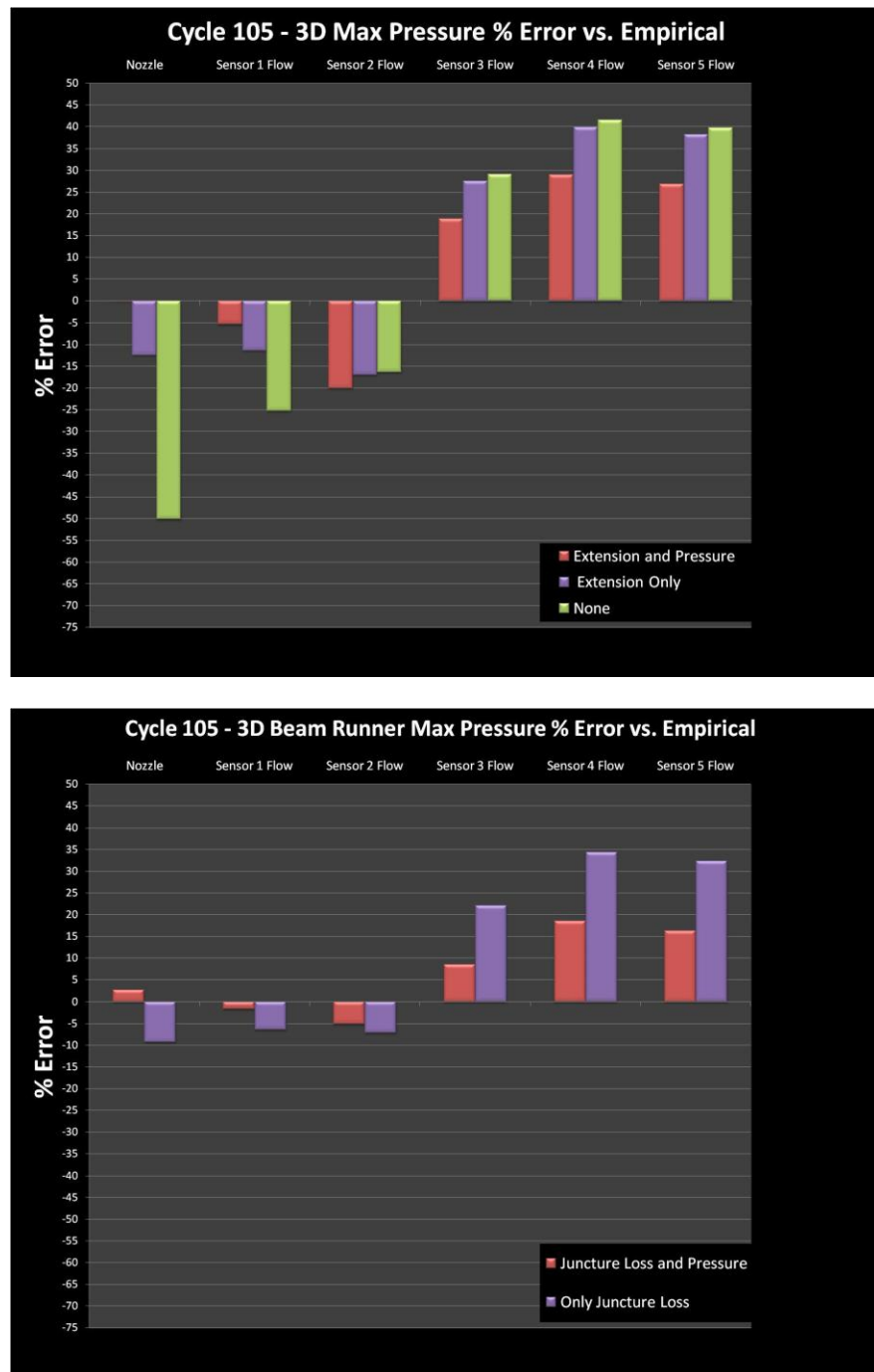
Figure 13 – These graphs highlight that modeling the feed system with beams in a full 3D analysis (bottom graph) can help improve the pressure drop through the feed system and in the cavity
