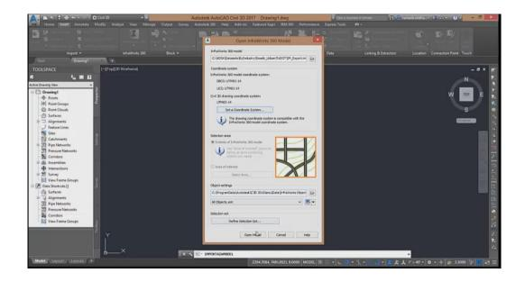
The terrain generated in IW 360 will now be visible in Civil 3D as a surface. You can use that surface as needed in Civil 3D.
