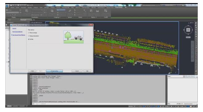
6. Civil 3D will generate a new surface from the processed point cloud data that can then be used in Civil 3D as needed.
