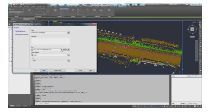
4. In the "Create TIN Surface from Point Cloud – Point Cloud Selection" dialog, provide the desired area or just leave the default, and click Next.
