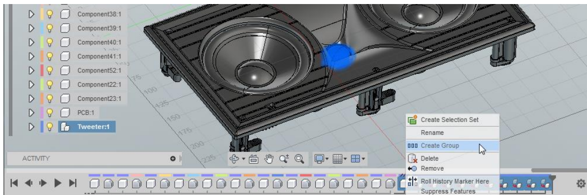
THE TIMELINE NODES FOR TWEETER ARE SELECTED AND RIGHT-CLICK MENU IS USED TO CREATE GROUP
