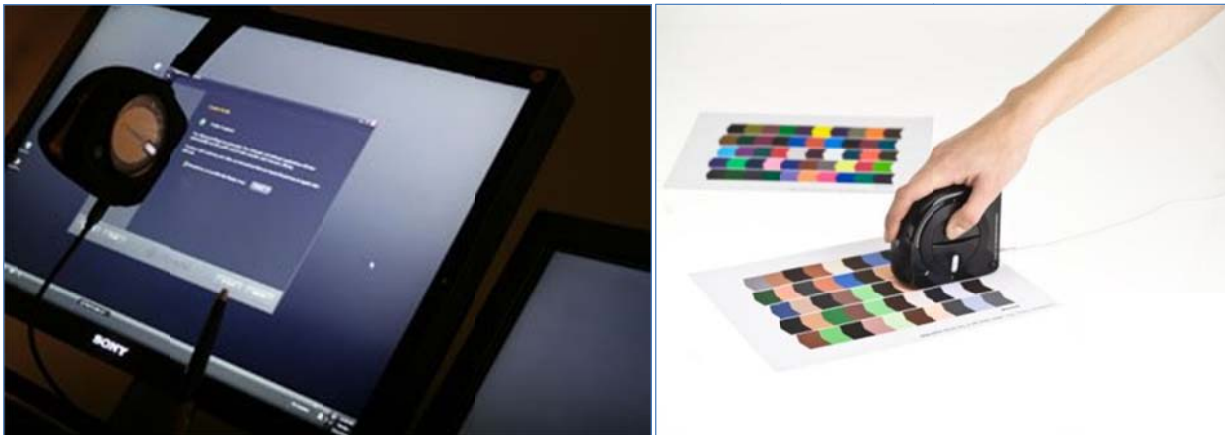
A portable spectrophotometer can define the response curve of your computer screens and printers.
