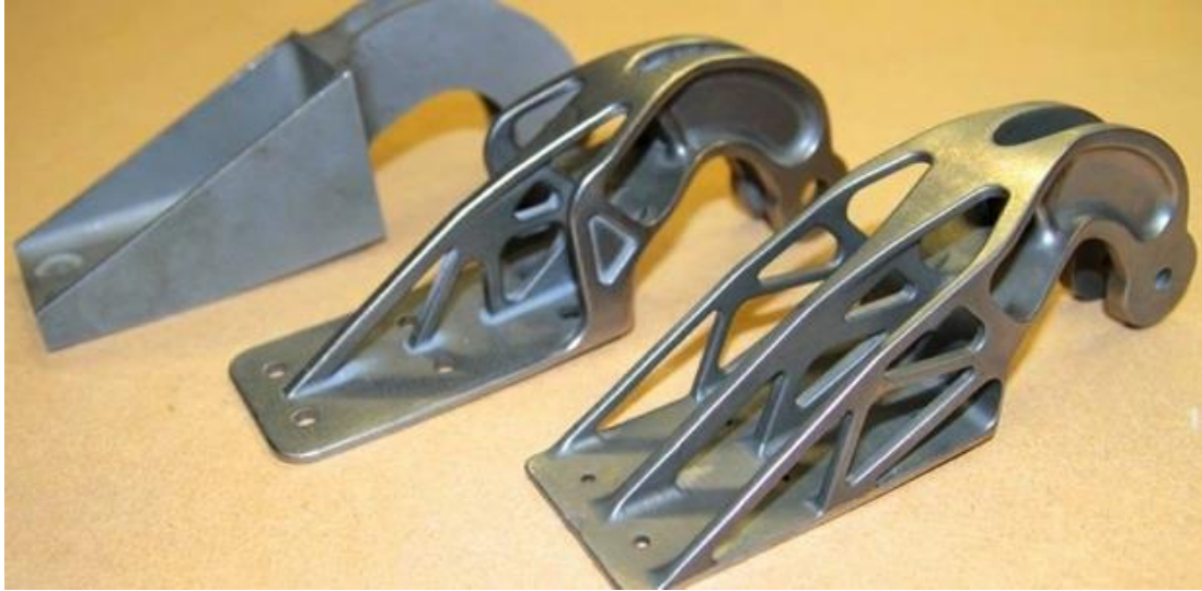
Metal parts 3D printed for European Space Agency (image from Engadget)
