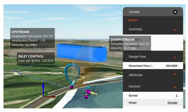
Of course you can manually create culverts and modify many aspects of their design including the layout as well as the shape, size, number of barrels, inlet configuration, and more.
