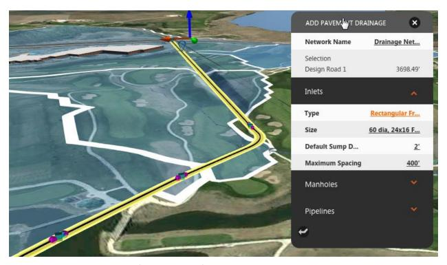
Or, you can do a combination of the two: let InfraWorks 360 lay out your drainage system automatically and then make changes, delete components, and add components to get the result you need.
