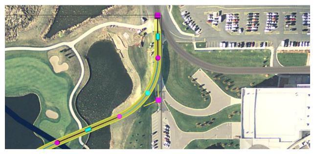
Something that Civil 3D can't even do, InfraWorks has gizmos (same idea as AutoCAD grips) located right on the road model, for both horizontal and vertical editing. When you change your view from top-down to more of an inclined view, the gizmos transform automatically and become PVI and vertical curve editing tools.
