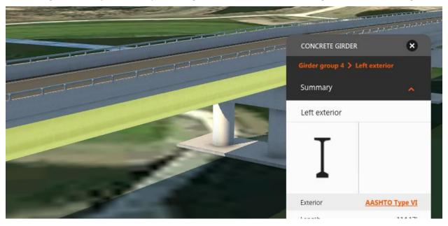
The same is true for piers, abutments, and even the piles underground. You can move, rotate, and even delete piers, you can change the configuration of the pier foundation, and you can even rotate and move abutments.
