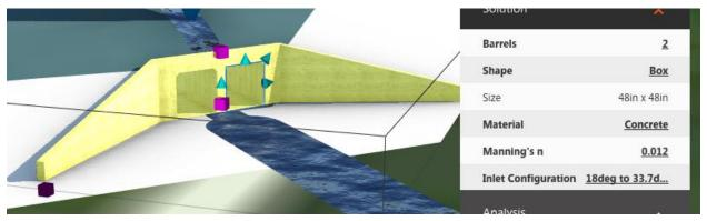
Pavement drainage is another feature set of Drainage Design for InfraWorks 360. You can create a system of inlets, pipes, and manholes for an entire design road or you can create the components individually using the tools on the drainage design toolbar.
