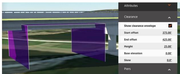
Another helpful tool is the clearance envelope which allows you to define the extents of an object that needs to pass under the bridge, and then assess or even make adjustments based on clearance.
