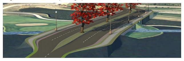
Another capability of design roads is that the tie-in slopes can be built according to a constant slope rather than a constant offset (that's what sketch roads to). This is much more representative of how roads are truly built.
