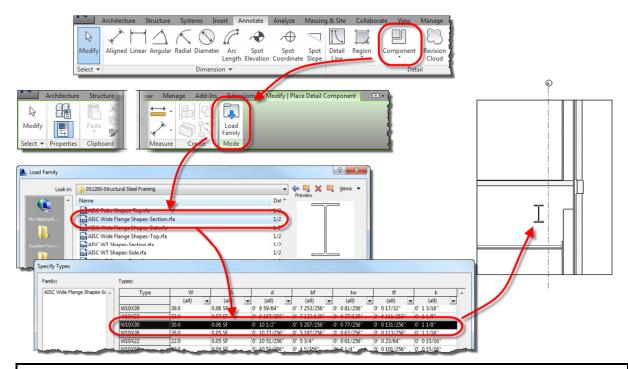
**Note:** It is important that you choose the "Detail Items" folder and not the "Structural Framing" folder. Items in "Structural Framing" are 3D model components. We would have used Families from this folder if we had decided to model the structural framing instead of simply represent it in the details.
