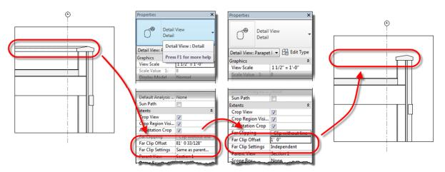
11. Navigate to the *Floor/Wall Connection Detail* Detail View and use the same process to turn off the Levels category and set the Far Clip Offset to 6".
