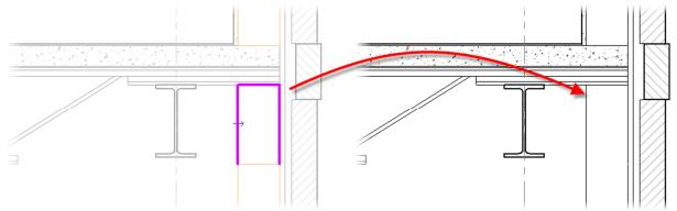
21. On your own, try to add the Detail Components for the 2'x2' acoustical tile ceiling as shown below (the notes are shown for clarification purposes only – don't add them to the detail). Refer to the following page for a few tips on completing this step.
