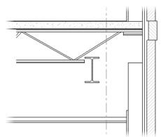
18. Align and lock the center of the beam to the column grid, and the top of the beam to the bottom of the bearing plate of the joist as shown below.
