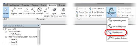
When you place a User Keynote, any Keynote that may be assigned to an Element or Material is ignored and can be overridden. The resulting choice is not applied to the Element Type or Material Definition.
