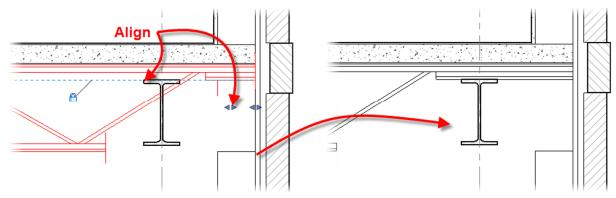
20. Use the **Cut Profile** tool to adjust the stud as shown below.
