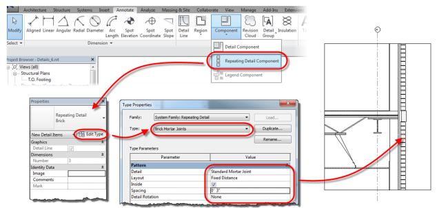
24. Repeat the process above to create the deck Repeating Detail Component using the settings shown below, then add it to the Floor as shown. Note that the Detail Rotation value is set to 90° Clockwise.
