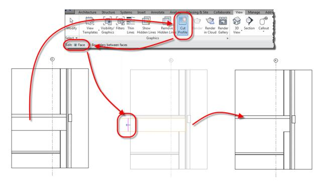
The bar joist Layer has not been deleted. It has merely been partly suppressed in this view. If you were to drag the right edge of the Crop Boundary to the right a bit you would see it. You can also select the sketch line of the Cut Profile and modify it or even delete it to bring the Layer back to full visibility.
