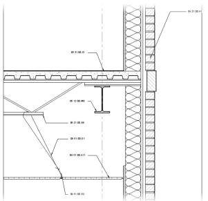
29. From the **Annotate** tab of the Ribbon, click the **Material Keynote** tool in the **Keynote** drop down menu. Select the Gypsum Wall Board layer in the Wall and place the note. When the Keynotes dialog box comes up, choose "Division 09 Finishes" then "09 29 00 Gypsum Board" for the Keynote to apply.
