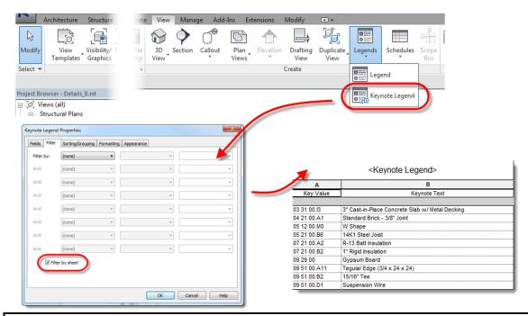
**<u>Note:</u>** Legend views can be placed on multiple sheets. The "Filter by sheet" option for Keynote Legends means that only the Keynotes that are actually displayed on the details on a given sheet will be shown in the copy of the Keynote Legend that is on that sheet.
