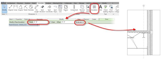
The detail geometry is substantially complete. While some of the line work line weights might need to be adjusted a bit, that level of development is probably best saved for later in the project. At this point it is time to add annotation. For purposes of this exercise we'll focus on Revit's Keynoting capabilities.
