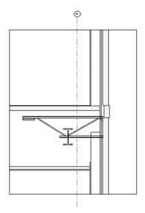
17. Select the bar joist, and from the **Modify** tab of the Ribbon, use the **Mirror** tool with "Copy" unchecked in the Options Bar to flip the Bar Joist around to the correct orientation and move it to the position shown below.
