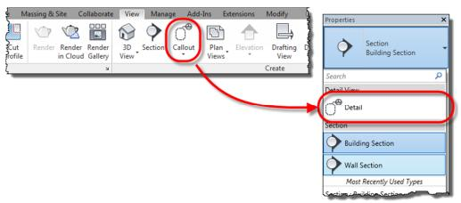
4. Place the Callout Boundary and Tag as shown in the following image. You can edit the Callout Boundary and Tag position by selecting the Callout Boundary after it is initially placed and editing the grips.
