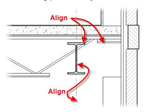
19. Align the Reference Plain in the bar joist that is at the grip locations shown below to the left edge of the beam and constrain it. (The grips will not be visible, however you will see the ghost image of the reference plane when you move the cursor across it and you will be able to select it).
