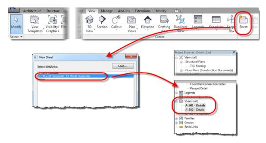
35. Navigate to the <u>A-501 – Details</u> Sheet and drag the <u>Floor/Wall Connection Detail</u> and <u>Parapet Detail</u> Detail Views onto the sheet, then drag the <u>Keynote Legend</u> Legend View onto the Sheet.
