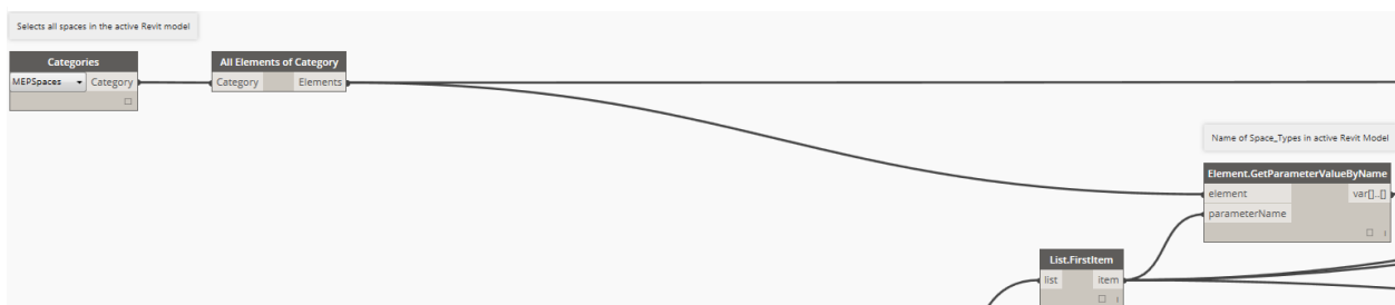
Figure 10 Access Revit MEPSpaces and read their Parameters
