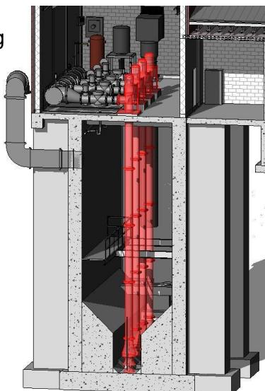
*"The purpose of an engineering drawing is to fully and clearly define what is required for a project. Without Revit, properly drafting the complex geometries associated with the wet well would have been a nightmare. In CAD it would not only have taken much longer, but we would still have been left with incomplete and ambiguous depictions of these complex geometries."*
