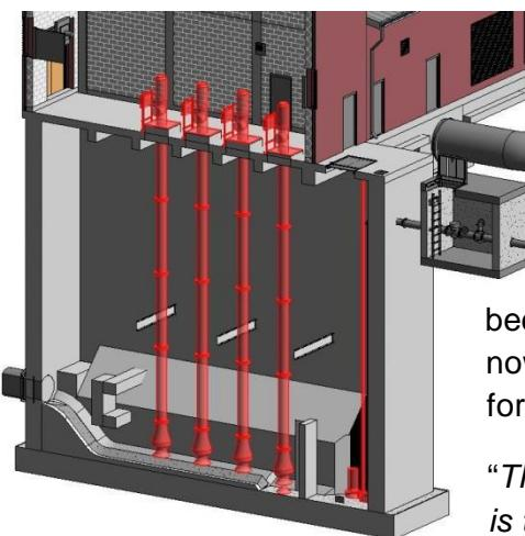
The project had several uniquely modeled families we created which include 4x45-foot long vertical pumps, sloped concrete fill, ogee ramp, flow splitter, fillets, anti-rotation baffle and a vortex suppressor. These families have been collected from the project and are now a part of the Process family library for use on other projects.
