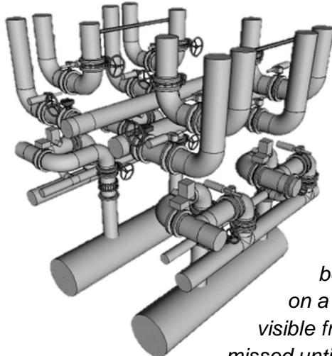
This project was originally done in AutoCAD MEP, and the vignette represents piping to and from four filters. This piping is typical for 2 rows of 14 filters long in a filter gallery, as well as the gallery on the other side of the building amounting to 52 filters total.
