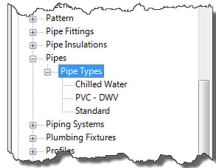
When making Pipe Types you will be combining the specific Piping System and the Pipe Segment, which should always be created first. There are 2 ways to make new pipe types, one is by using the Project Browser and the other via the Properties Palette. Below is the example of using the Properties Palette:
