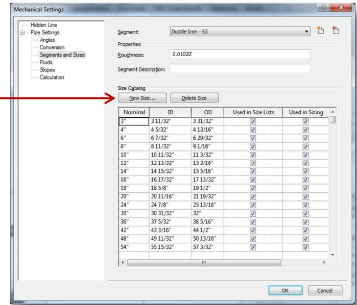
Now you can delete the remaining size(s) left from the default pipe segment you started with. Continue the above process for all needed pipe sizes for the new pipe segment.
