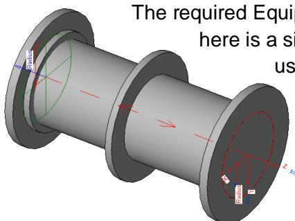
The required Equipment will most likely need to be created. The piece shown here is a simple wall casting family we needed to create. It was created using 2 cylindrical extrusions (one for the pipe and one for the cuff), 2 flanges and 2 pipe connectors. Content can be as simple or as complex as you want to make it. We believe, simple is better.
