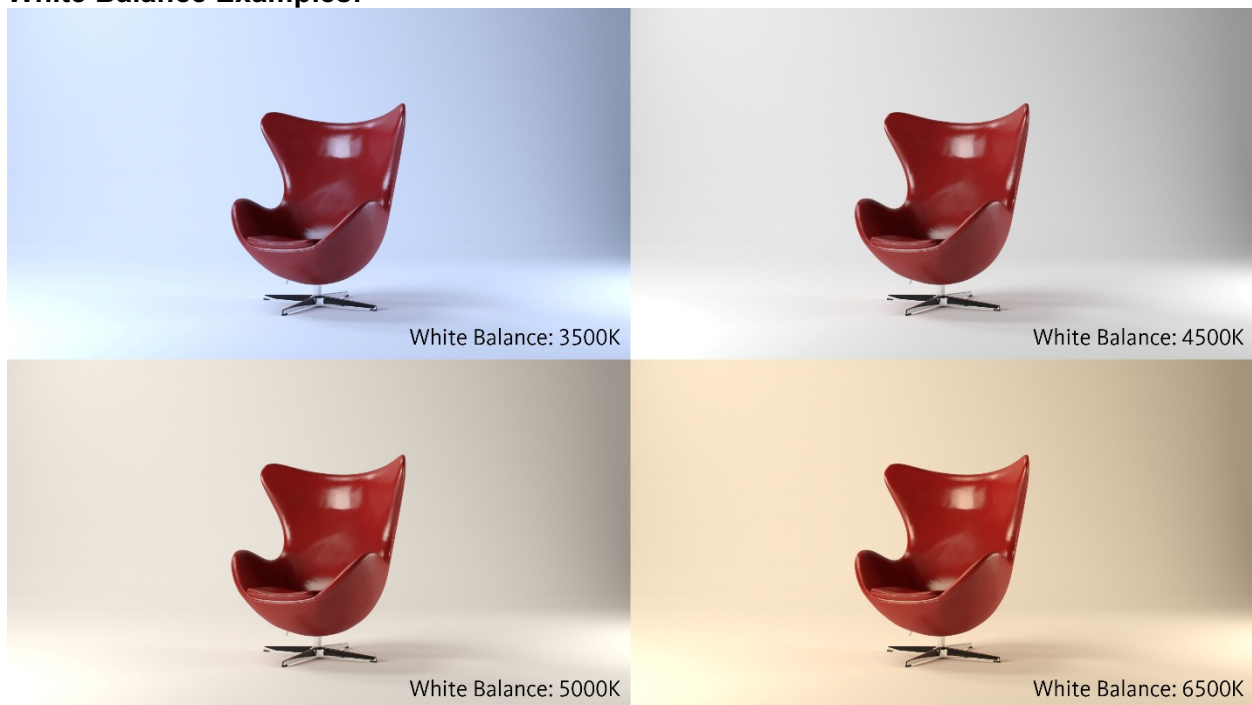
IMAGE 4-18: These renderings show the difference White Balance can have on the rendering. Note that the lights are set to 4500K, this is why the rendering with a White Balance of 4500K appears to have “White” light.
