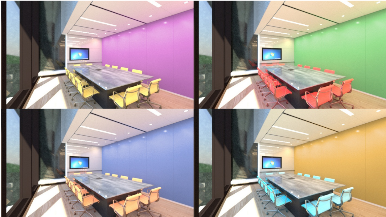
IMAGE 7-2: The combined LPE's above generate the Beauty Pass, and then can be altered for an infinite amount of color variations without ever having to re-render the image. This can be extremely helpful when studying color options for finishes, etc. Since the LPE's show all the rays that bounce per pass, the color adjustments will show up in the bounce lighting and reflections!
