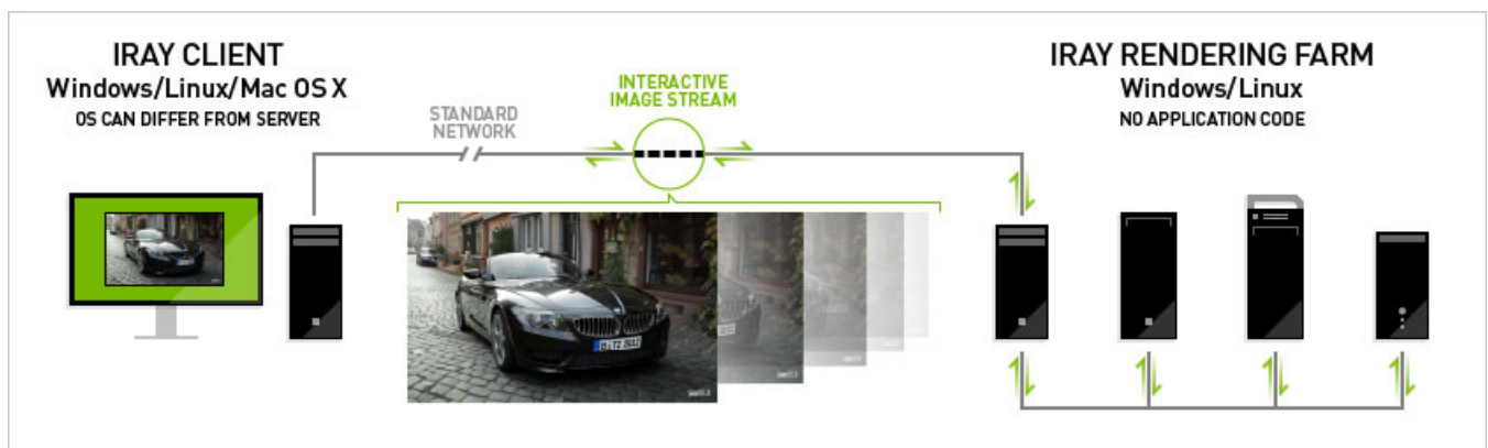
IMAGE 8-3: This diagram shows how Iray Server works across a network. (Provided by NVIDIA).
