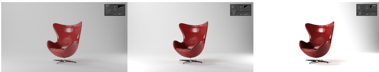
IMAGE 14: These renderings illustrate the differences in the Image Control. The center rendering is with the default settings. The left rendering is completely set to 0, and the right is set to 1.0.
