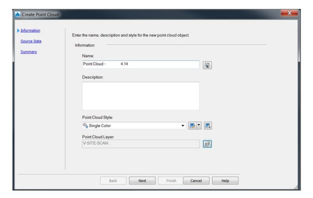
Choose the Point cloud data Create a new point cloud database Click on the plus sign And navigate to the file and open Then click next
