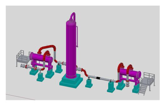
Notice in the properties of the Valve Line Number Tag and Tag are transferred from the P&ID Description and Facilities Item Number are transferred from the Catalog and Specs
