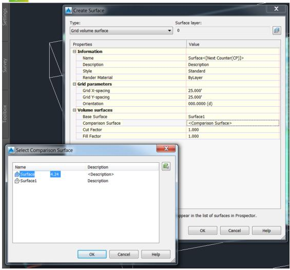
There will be a Surface created of the difference between the two surfaces The result is the surface below the original Surfaces
