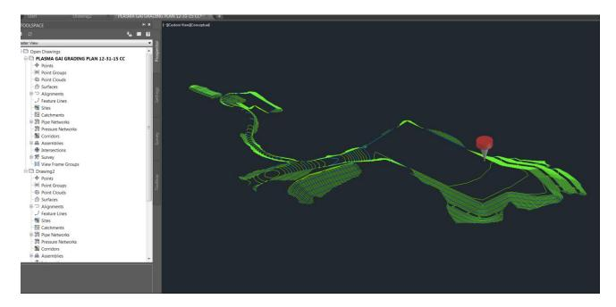
You can either create a surface from the ribbon or in tool space In the Home Ribbon in the Create Ground Data Tab Click on Surfaces Create Surface
