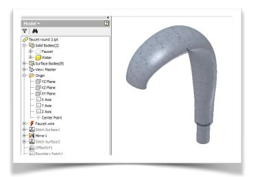
4. If Solid Bodies were used to create water volume then use Make Components to create an assembly of faucet and water volume.
