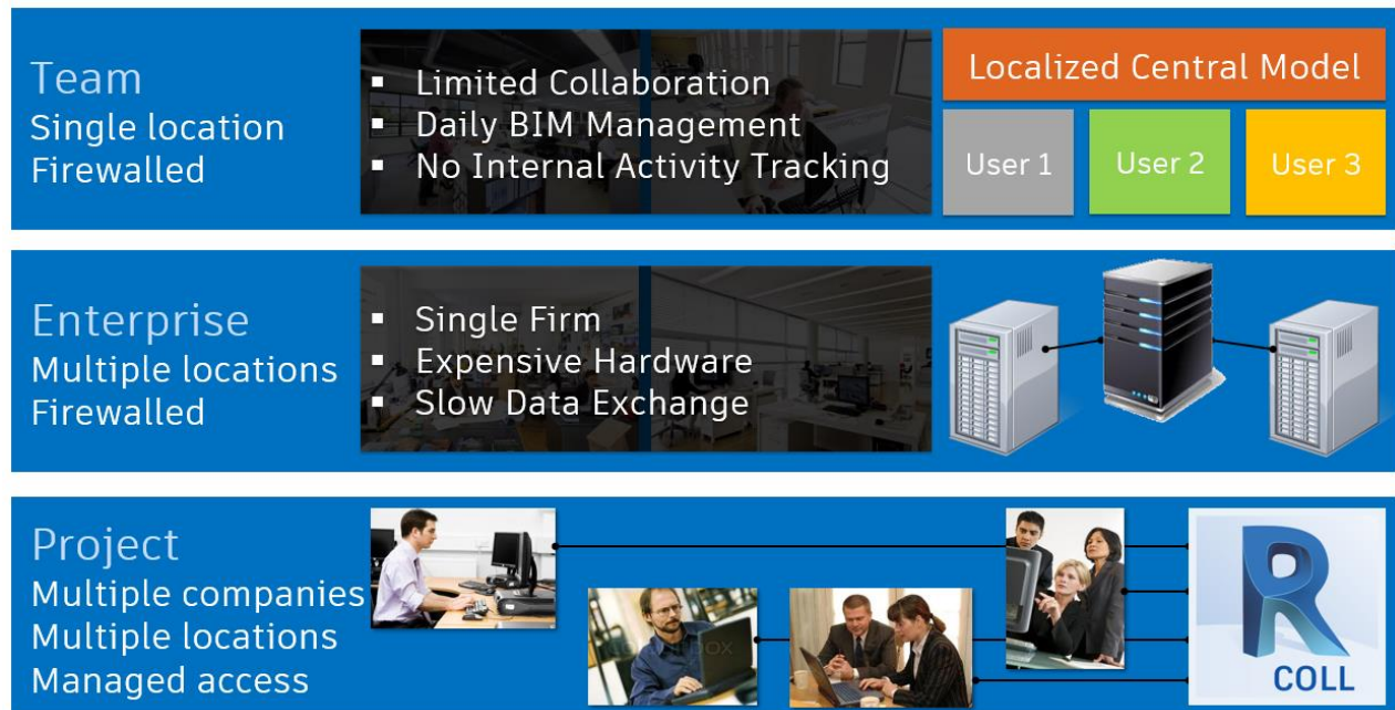
Figure 6: The three phases of Revit worksharing
