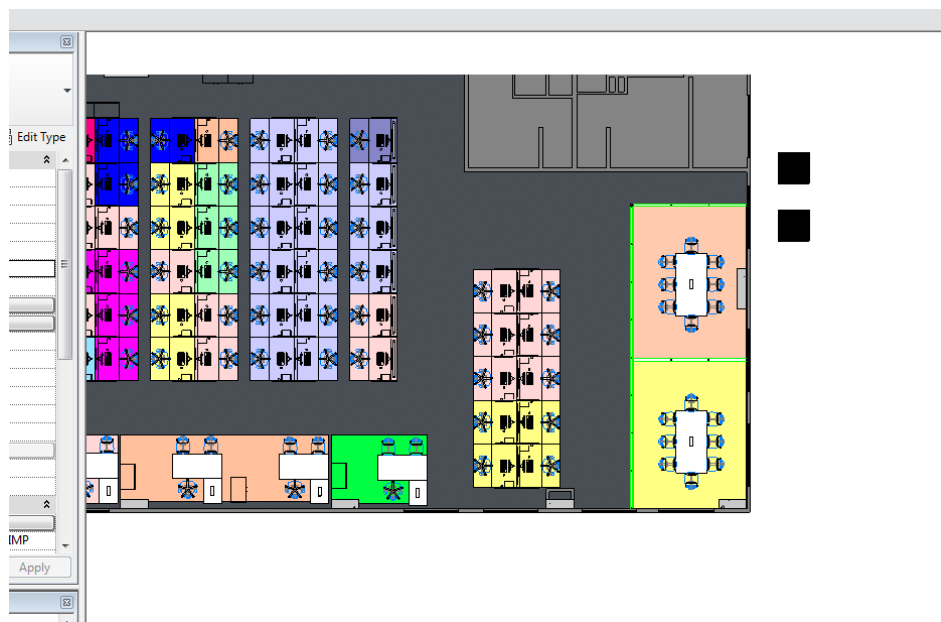
Fig. 11 – Plan view with furniture using visibility filters from schedule key department values
