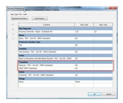
Routing preferences contain information about material type, fittings and flanges. Each of the settings allows the user to set a size range for the segment. In the event that an additional fitting type is "allowed" in all segments, the first listed fitting is used by default.
