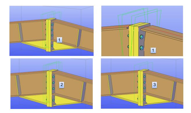
→ Conclusion: Revit exports shortenings that are recognized and used in Advance Steel, but will lead to problems for a lot of steel connections as they use their own shortenings that will overlap with the existing ones from Revit.
