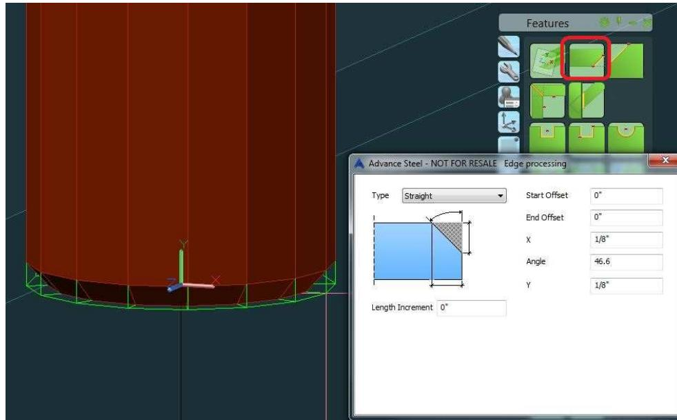
! Rotate to front view using the view cube / Use the “UCS view” command from UCS tool palette
