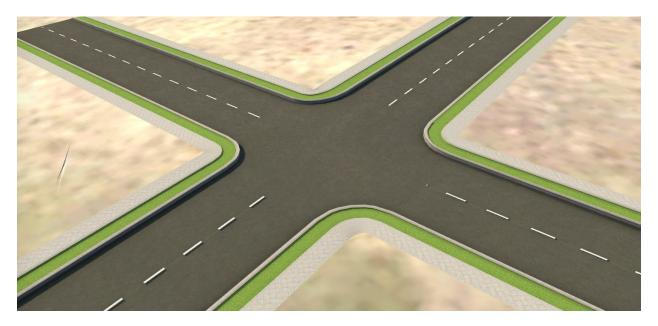
This intersection will not be able to be designed per a design vehicle's turning radius, nor would dedicated turn lanes be easily created.
