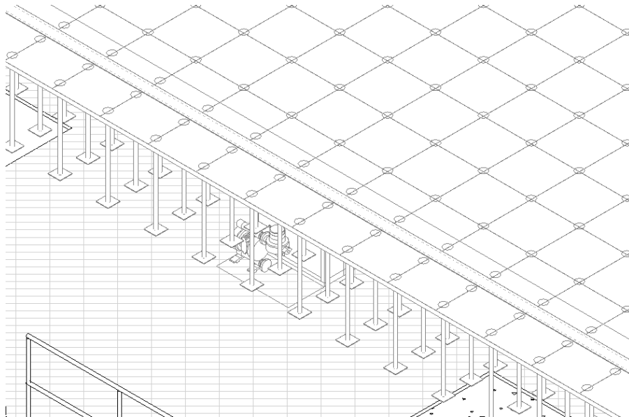
ARCHITECTURAL DESIGN MODEL M+W RAISED METAL FLOOR WITH SUPPORTS
