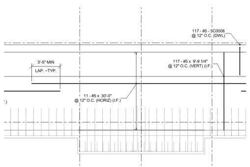
REBAR SPECIFIC TOOLS USED TO CREATE SHOP DRAWINGS IN REVIT
