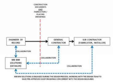
TYPICAL SHOP DRAWING PROCESS VS. INTEGRATED APPROACH
