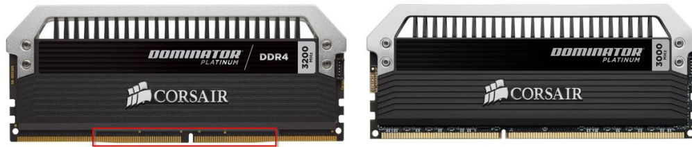
DDR4 DRAM (left) and DDR3 DRAM (right). Image courtesy anandtech.com
