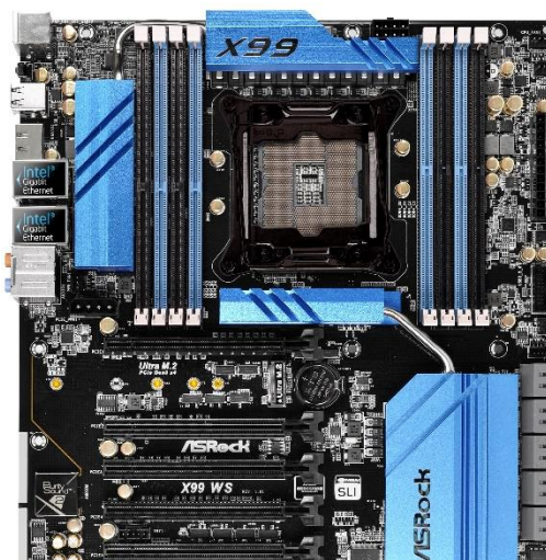
An X99 motherboard with 8 slots with a color coded pair of four channels each. Install 4 DIMMs in one colored set of quad-channels, then 4 DIMMs in the other colored quad-channels. Refer to the motherboard manual for memory DIMM compatibility and installation instructions.
