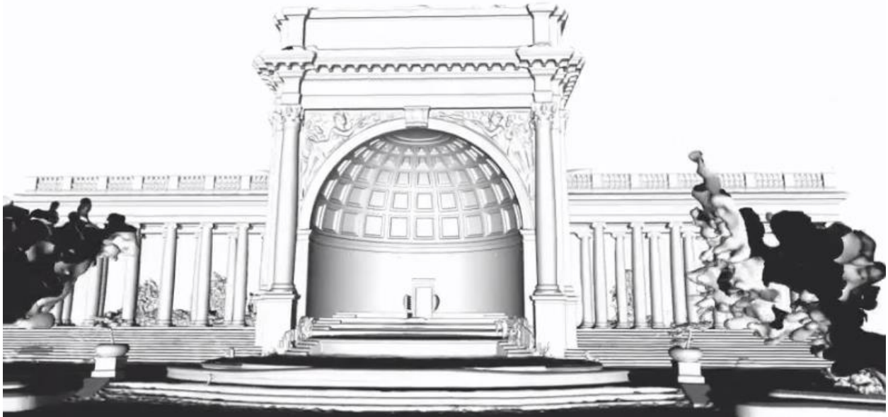
MESH CREATED FROM RECAP 360's SCAN-TO-MESH SERVICE
