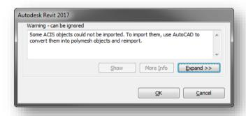
Note, DWG Sync will bring in any External References that are attached to the original DWG file, regardless of the attachment type (overlay vs. attach.) If the exclusion of External References is desired, they must be unloaded inside the original DWG file before using *DWG Import*.
