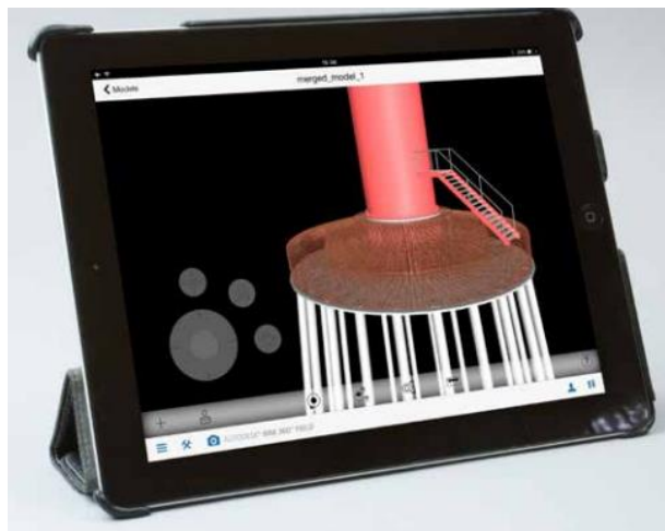
BIM360 MODEL FOR USE ON-SITE OF WINDMILL FOUNDATION REINFORCEMENT
