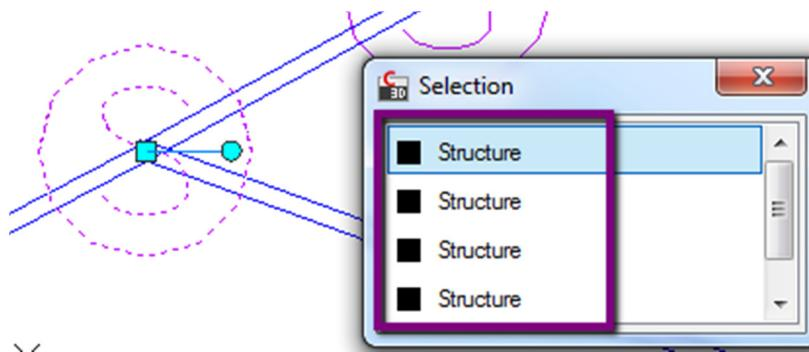
duplicate and sometimes more (depending on the amount of pipes coming into the structure) structures created. This could cause quite the headache to determine the correct structure, created from the actual SHP data, and the one that was put there by Civil 3D on account of the pipe start or end.
