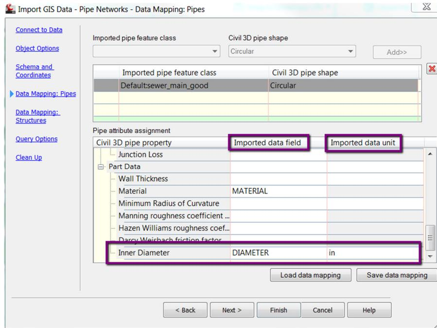
Beginning with selecting the Imported Pipe Feature Class, then the Civil 3D Pipe Shape. The pipe shape selected here will correspond with the parts lists selected in the Object Options. Now the properties from the object data must be matched up with the part properties from the Civil 3D Parts List.
