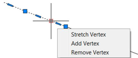
These options make quick and easy work of the vertexes and will preserve the proper inverts per the original object data. If these are really unnecessary vertexes, then removing them will not alter the slope or invert object data attached to the objects, everything will remain intact and correctly import. Please note that to edit this data in one of the above options; it will need to be imported via MAPIMPORT, cleaned up, and then MAPEXPORT back to SHP.
