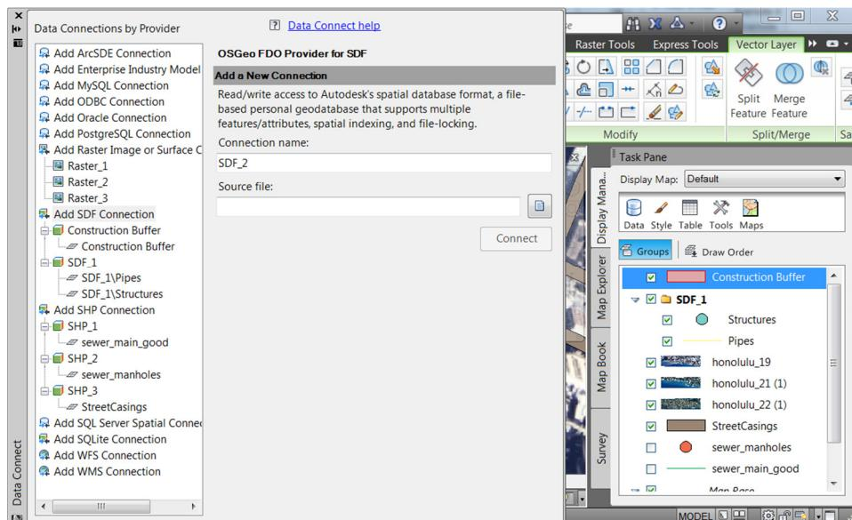
Now that we have our pipes in Map 3D we can illustrate an example of an analysis to make sure we have the desired setbacks around the proposed pipes in order to start construction. Using Map 3D's buffer tools will make quick work of this.
