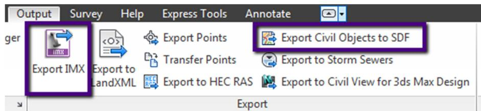
Next we will want to export out the pipe networks via IMX. This is found within Civil 3D via the OUTPUT tab>EXPORT panel or the IMX\_EXPORT command. Again running this command will populate a dialog that will write out a IMX file for import into AIM.
