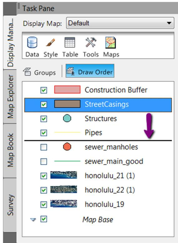
Also notice the check boxes by the different layers. Checking or unchecking these will also maintain the connection, but control whether or not they will be displayed.
