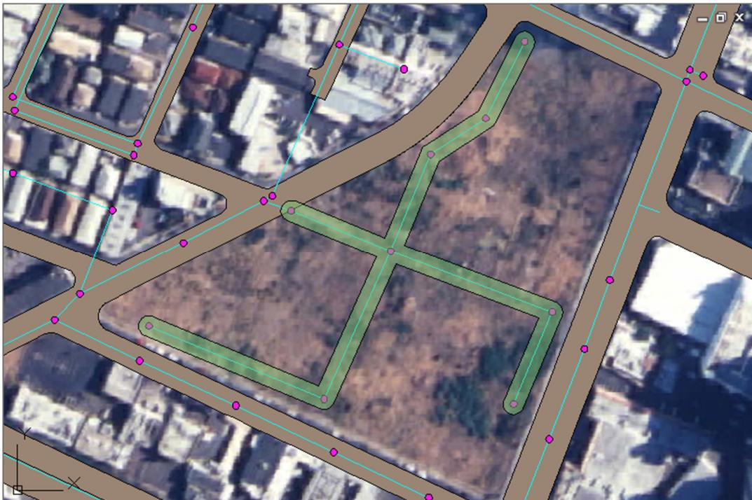
Since we have models built in all products this new buffer now in SDF form can be easily imported directly into Civil 3D to see how it impacts surrounding utility locations and new design. It can also be attached in AIM and sent to the cloud to use on site as well as to get a real world feel on your desktop.
