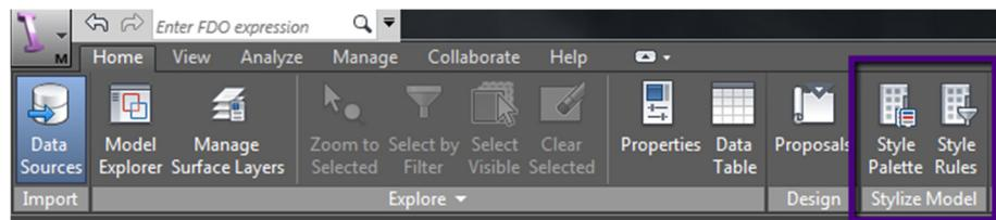
Starting from the HOME tab, under the STYLIZE MODEL panel, we will select the Style Rules button. Up pops the Style Rules dialog box. Here each feature will have its own tab to assign options to stylize. Since we are concerned with the pipes and pipeline connectors we will select these tabs.
