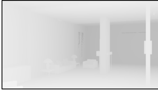
Z-DEPTH RENDER ELEMENT USED AS A MASK FOR DEPTH OF FIELD BLUR
