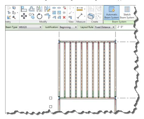
Now we will place secondary steel in the other bay on level three. This time the spacing will be 4 feet with the same section. Once complete the structure looks like this in 3D:
