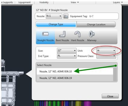
If the ADSK model has flanges, select the appropriate end type and rating (150#)
