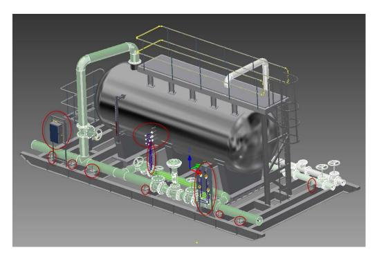
We will suppress the control panel, the instrument panel, piping clamps and instrument taps and piping. Right click on the control panel and select 'Suppress':
