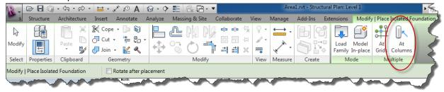
3. Window the MAIN columns (at the intersections of the grid), then select 'finish' – make sure you do not include the stairs supporting columns:
