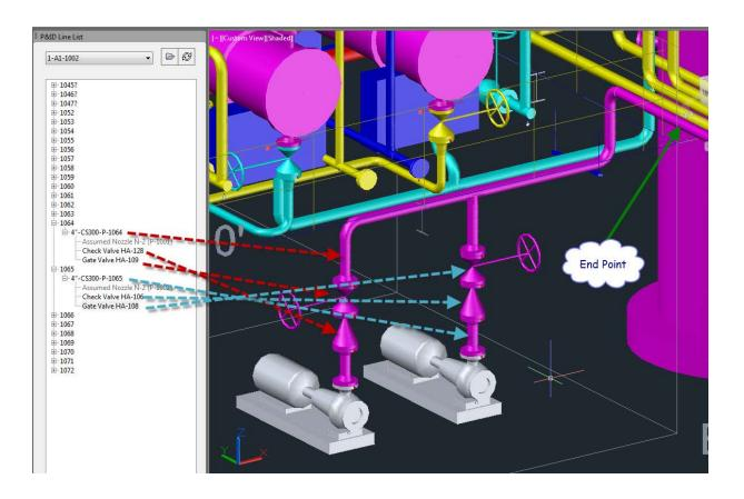
2. Optional – add 3/4" drains to the lines you just modeled. The spec CS300 branch table is set to automatically place a threadolet. You can then place a 6" pipe or a 3" nipple – select the nipple, gate valve and plug from the piping spec palette:
