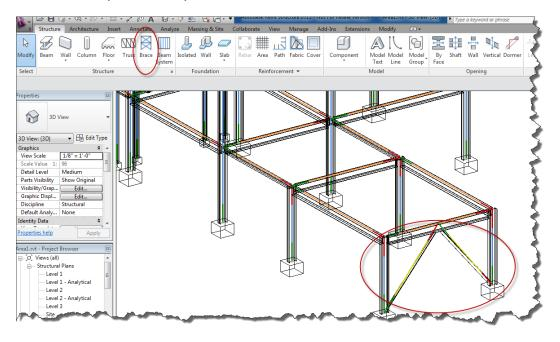
Save the project and let's demonstrate Steel Detailing. We do this by transferring the model to AutoCAD Structural Detailing. Again using the Extensions Ribbon, simply select the AutoCAD Structural Detailing >> Steel Detailing Link command. (**Tip** – Open ASD before you execute this command):
