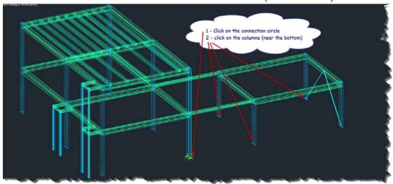
4. Now we will do the Beam to Column connections. There are many different types of connections depending on whether it is a beam to flange or beam to web connection. We will do a simple example. Select the end plate – Beam/Column flange connection:
