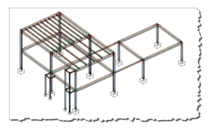
Finally (optional) we will place bracing using angle section L4x4x1/2. Use the command 'Brace' in the Structural ribbon. (Hint – keyin 'S' then 'E' to snap to the bottom of the columns and 'S' and 'M' to snap to the midpoint of the beam. The result will be:
