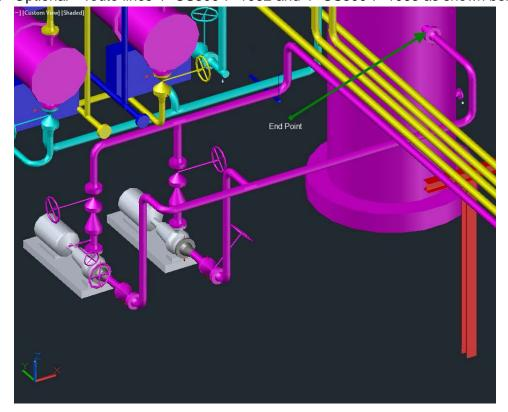
Place a 3/4" threadolet on the bottom of the eccentric reducer and then replace the
