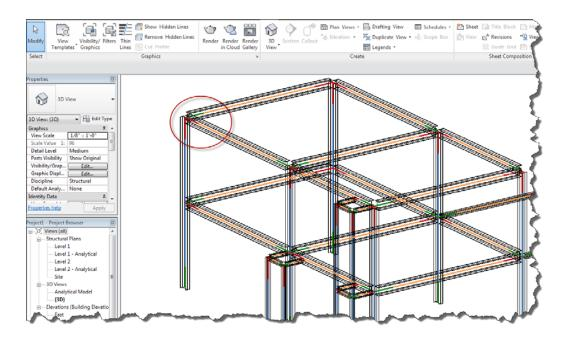
Note that the beams are placed by center and not by top-of-steel. This can be corrected very quickly as follows:
