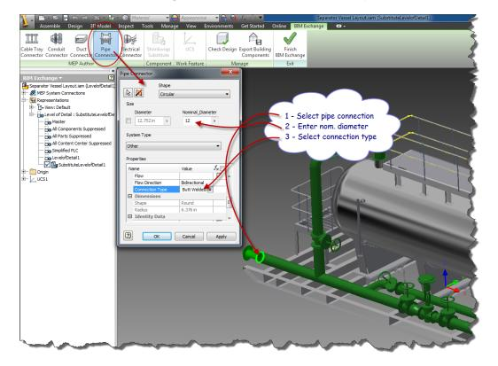
The nominal diameter should be rounded down to the appropriate diameter (12" and 8") and the connection type should be set to 'butt welded' in the properties section. Do this for all the pipe ends.
