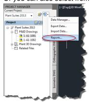
Using the AutoCAD Plant Report Creator 2013 – select the project and then select the extended Equipment List:
