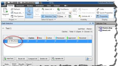
b. Give the test a name 'Pipe vs Structure':
