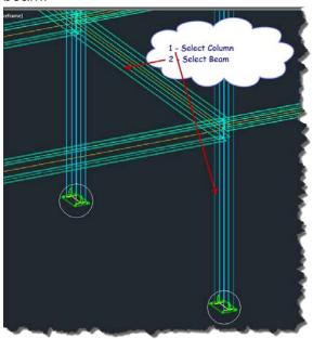
5. In the connection dialog box select the default values but in the stiffener tab, select a triangular stiffener under the connection and remove the ribs in the column. Apply will show you a preview and OK will place the connection:
