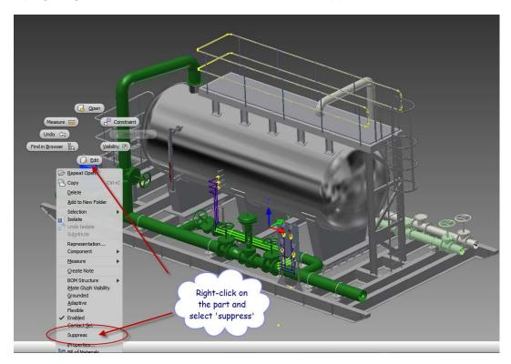
Repeat this for the piping clamps and instrument panel. Instrument lines are suppressed differently because the Inventor module is not in the suite:
