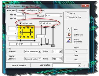
3. Click OK and after the connection appears, we can copy this onto the rest of the main columns (Note if the circle around the connection is too large or too small to be visible, reset the size by clicking on Preferences >> Structural Detailing>>Steel>>Connections and setting the size value to a suitable size):
