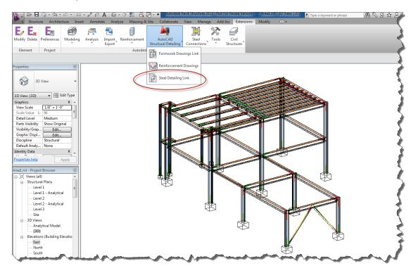
Select the option to 'send model to AutoCAD Structural Detailing'. The process may take a short while, but once complete ASD will be opened and the model can be viewed in ASD.
