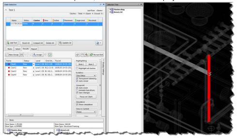
f. Click on each clash listed to review each clash. There will be two clashes that are real and two that are due to the supports being attached to the structure. You can ignore these by selecting 'Approved' in the pull-down under status:
