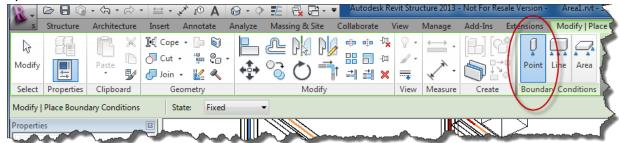
select the ends of the columns (click on the green lines) and the boundary points will be place. Click <esc> to end placement.
