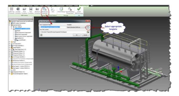
Select the correct template in order to ensure the correct UCS is used for Plant 3D. The correct template is 'Standard (DIN).ipt' in the 'Metric' tab, which can be found by clicking on the icon alongside the template pulldown. Click 'OK' to start the shrinkwrap process.
