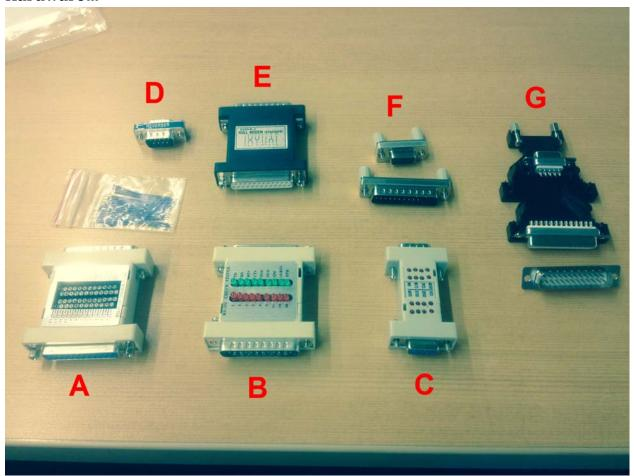
A = DB25M / DB25F Wiring Adaptor / Jumper Box
