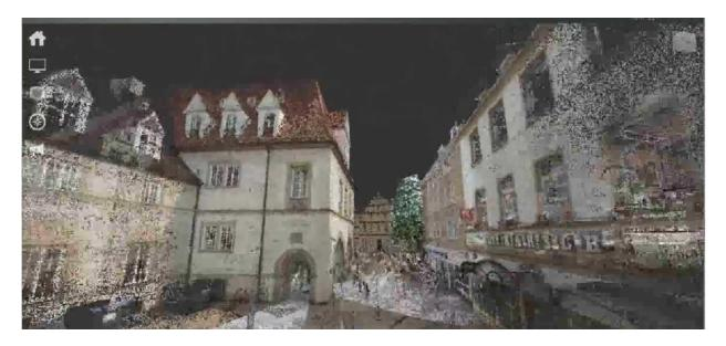
• Creation of As-Built Models, Using Laser Scan Data Alignment
