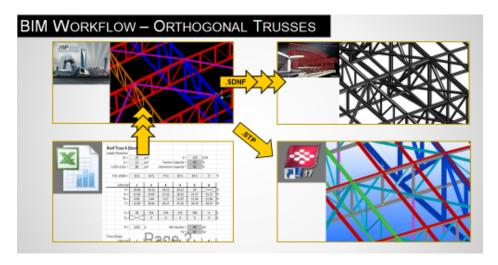
What we were trying to achieve for the Orthogonal Trusses project was to be able to easily update the geometry and structural load properties within the analysis model. We chose to modify the joint coordinates and the loading criteria of the structural analysis model via the interactive database of SAP2000. We were able to export the SAP model to SDNF and import that into Revit. This transferred the geometry and the structural section properties to the documentation model.
