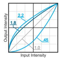
Numbers less that 1.0 de-gamma correct an image, *normalizing* it back to gamma of 1.0. Numbers greater than 1.0 add gamma correction, brightening the image.
