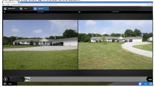
At the bottom right, just above the "Next" button is a Ruler. That is very important. ReCAP does not know the scale from the photos. It needs some reference points and a reference distance. Click on the first point on the ruler, go to the left image and select an existing point. That point number now appears in the ruler. Now pick a second existing point in the left image. That point's number appears in the second slot. Type in the known reference distance.
