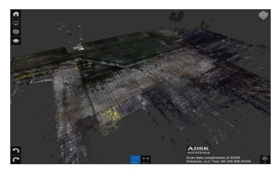
In less than 48 hours, 3 different laser scanners were used to perform 180 individual scans. Scans were registered in the field as scans were performed. Three registered point clouds were created and completed within 10 minutes after the final scan in the facility. The image below was the only as-built data that was available for the plant.
