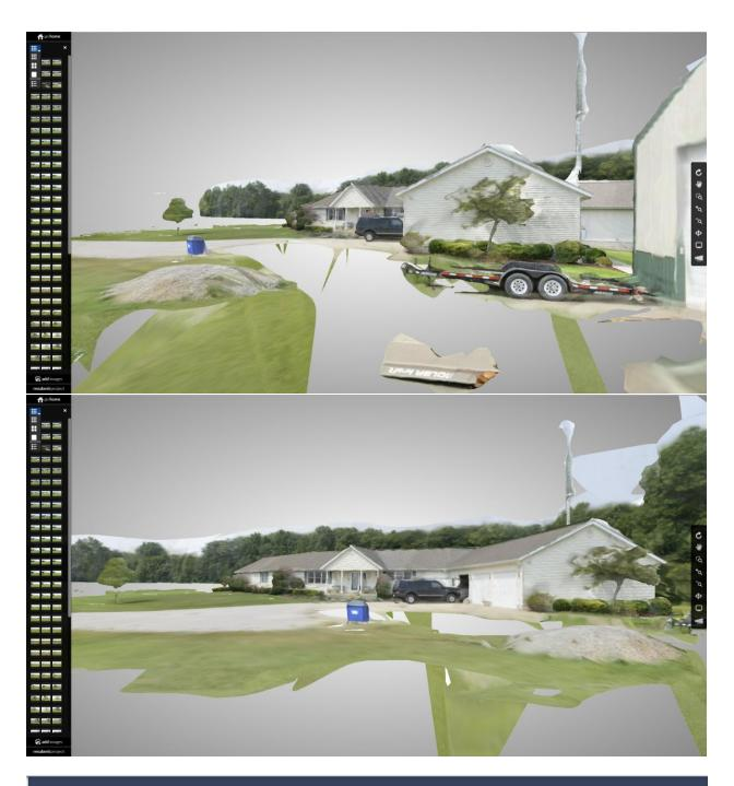
This is a proxy mesh with only 200k triangles. To access the full resolution mesh (10.34m triangles), download the OBJ, RCM, or FBX
