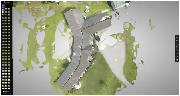
I can use that in Revit! Import the RCS point cloud file. Then trace the point cloud.
