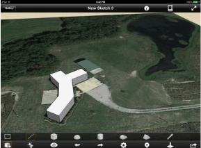
Switch to Top Plan view, so we can add lines to mid-point making the roof ridgelines.
