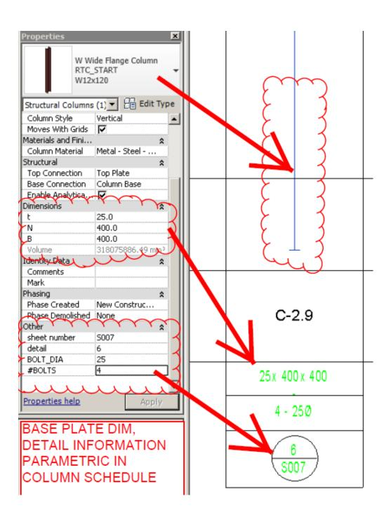
13. Tag the new column and move the new parametric tag boxes into place. They should snap into place. The final text box should look like the image above.
