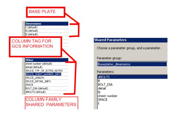
Open the family parameters and notice the difference types of parameters already created as shown above. All the parameters are shared parameters so they could be shared between the column family and the column tag that will both be displayed in the GCS.
