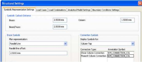
Control the width of the splice by the following setting in the "manage-structural settings" properties box. Note that only the top of the column will be adjusted the bottom of the column will remain at its modelled location.
