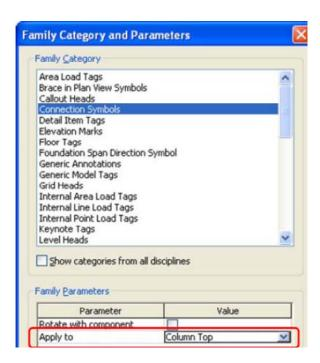
Load new connection type in "Structural Settings under "Symbolic Representation Settings"
