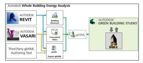
Whole building energy simulation measures expected energy use (fuel and electricity) based on the building's geometry, climate, building type, envelope properties, and active systems (HVAC & Lighting). It takes into account the interdependencies of the building as a whole system, so it is a particularly useful way to "keep score" as you work to reduce building energy use.
