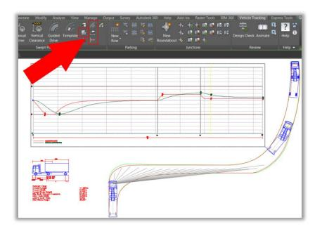
Although there is a dedicated wizard to alter the path styles, you have more control and flexibility over the styles by selecting a path and editing via the Vehicle Tracking properties button on the right of the ribbon.
