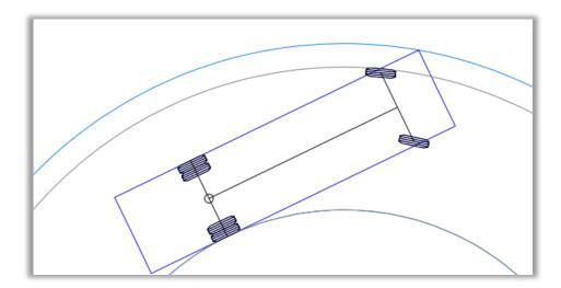
The front of the vehicle above (looking at the outer, blue body envelope arc plus the outer, grey chassis envelope line) will be affected mostly by the speed of the maneuver and the turn rate restriction that is applied.
