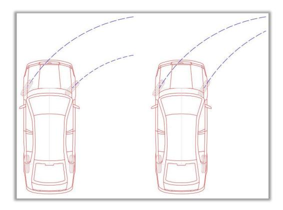
Note how the non-Ackerman geometry on the right example would create tire scrubbing, limited grip and so probably a larger turning circle and the 2 wheels would eventually try to cross each other's path. The example on the left illustrates how the Ackerman steering setup allows the inner wheel to turn at a greater angle.
