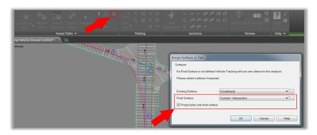
In most cases, for swept paths you actually only need to specify the Final Surface; the Existing Surface is used for designing roundabout corridors in Vehicle Tracking, when there is a need to tie into existing ground. Also, ensure you select the check box entitled Project plan onto final surface; this will ensure that your swept path is located on top of your surface and 2D lines are draped onto the surface for presentation and ease of modeling.
