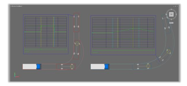
The truck on the right has a much more calm and realistic maneuver, note how the graph illustrates much more gradual changes in steering angle along the green line. The downside of this realism is that much like real life the vehicle becomes less maneuverable. Now imagine trying to drive a site that had been designed without transitions applied, it may be acceptable for very low speed parking scenarios but it is generally not advised.
