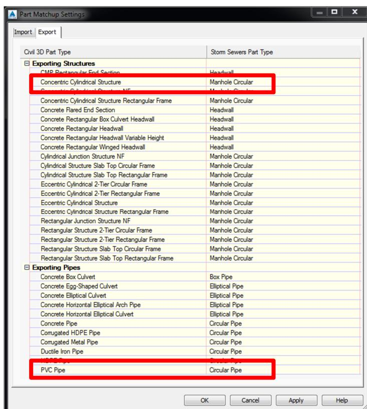
Exporting the Pipe Network is handled from the Analyze tab in the ribbon menu and selecting Edit in Storm and Sanitary Analysis.
