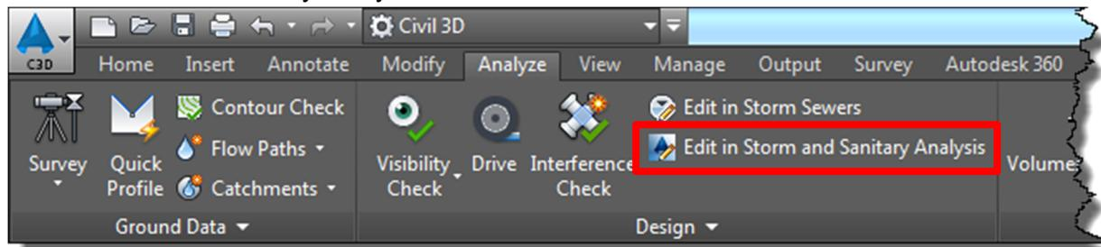
Select the Pipe Networks to be included and create a New Project when SSA launches.
