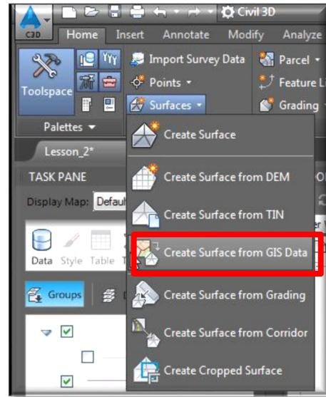
Be certain to determine which property in the SHP contains the elevation data to be used for creating the surface. One simple way is to attach the SHP, highlight one of the contour lines and select Properties. From the Properties window a list of the properties will appear that are a part of the SHP and allow you to determine which one has the needed value for contour elevations.
