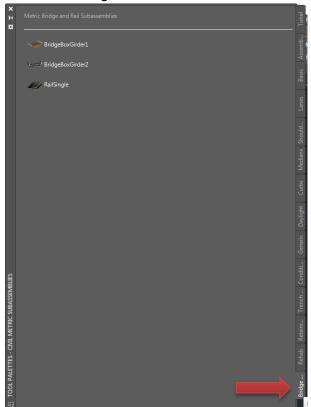
6. Then, select the subassembly named *RailSingle* and insert it in the center of the *Assembly*.
