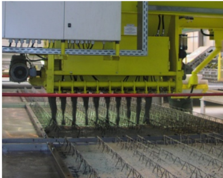
Concrete spreader fills in the concrete
