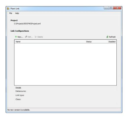
First we click on "New..." To start the wizard of PlantLink. The first thing we need to do is select the database. For this example we select the ProcessPower.DCF file which is the AutoCAD P&ID database.
