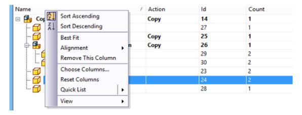
As users make changes to the configuration, the main grid "Name" value changes to preview the new component name, users can add the "File Name" column to see source file name or use values like <u>Component ID</u> and <u>Component Quantity</u> help to track source file behaviors.
