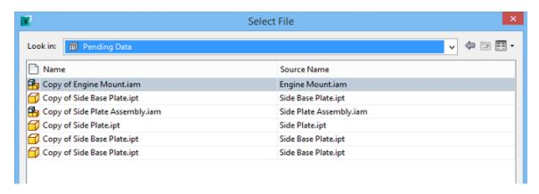
Once referenced into the operation Vault will create the new file and rebuild the new structure with the selected file like it would with any normal replace operation.
