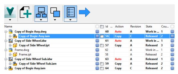
In drawing mode though, users can now set design documents to copy independently of the model and specify new file names and save locations, allowing greater flexibility with the copied output.
