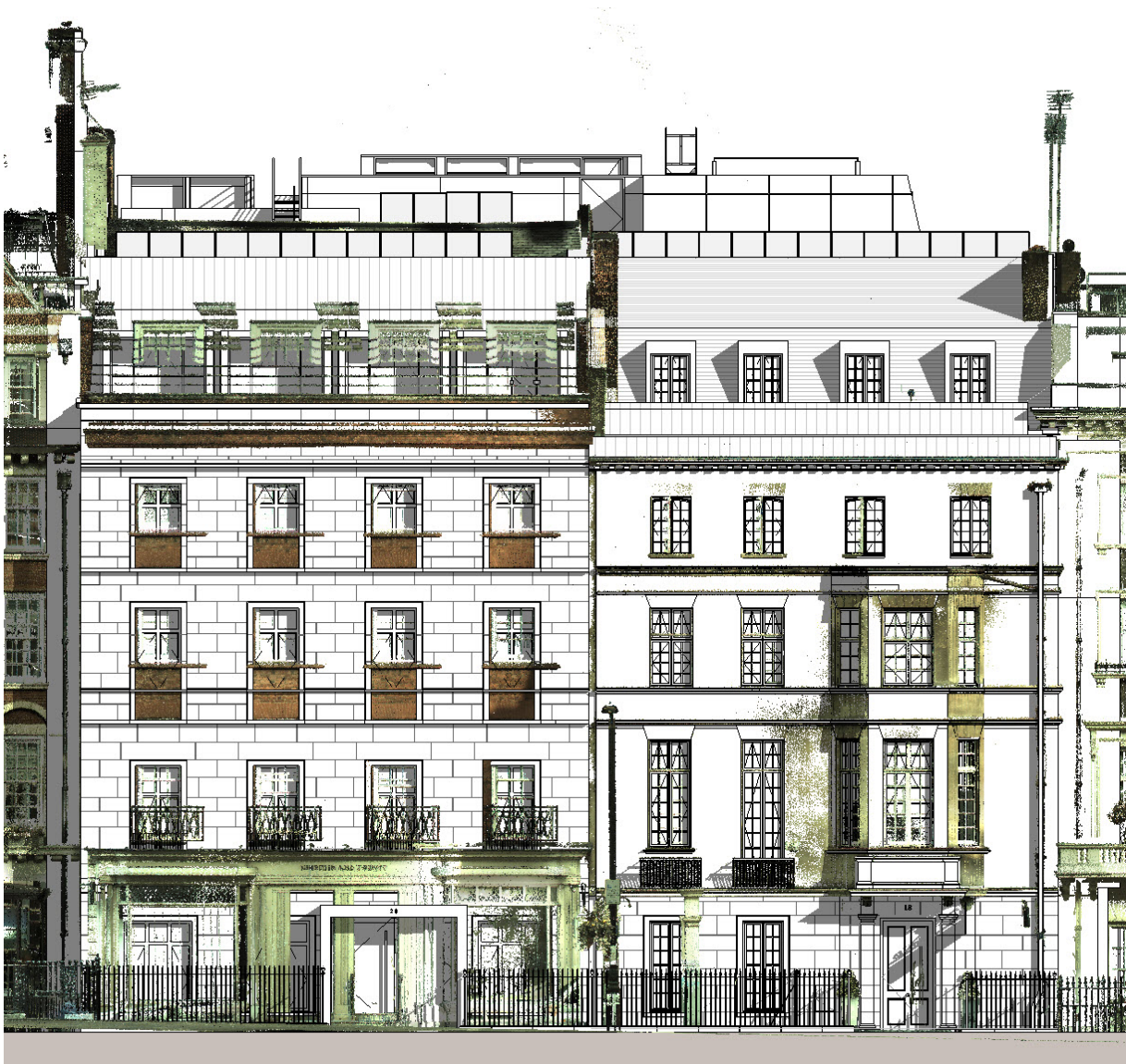
Grosvenor Street Elevation (Point Cloud overlaid Autodesk Revit Model)
