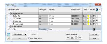
• The new parameter is created with an option to select "True" or "False" in the equation column. This parameter currently does not have a related rule associated with it, so modifying the value will not have any effect on the model.
