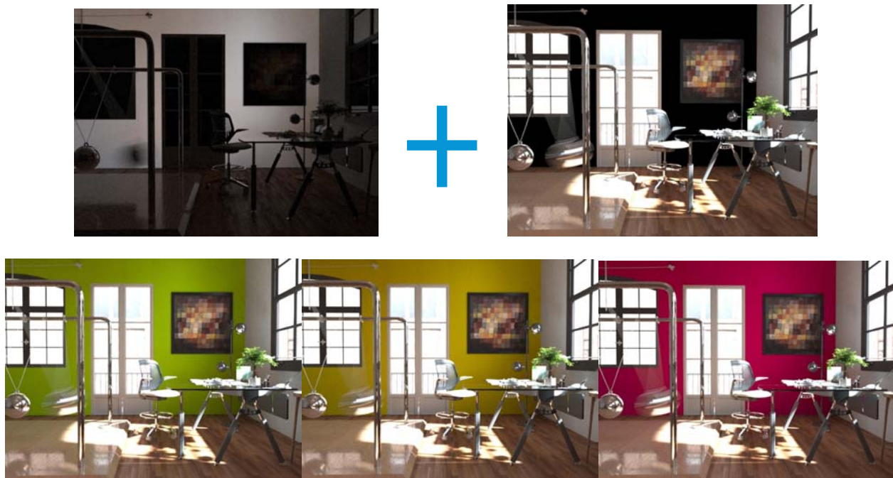
IMAGE 8-1: This shows LPEs in action. The first image is just the rays that hit the white wall, while the second image are all the other rays in the render. When compiled, you can change the color of the wall in post-production without re-rendering! (Images provided by NVIDIA)
