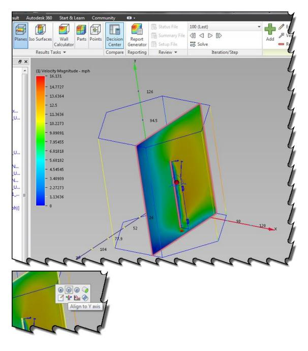
Adding Planes from the Results tab using the "Add" button in the ribbon will generate a default plane in the model witch provide insight. Left Mouse click on the plane to adjust orientation, using the arrows to slide its location.
