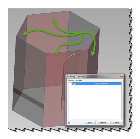
Lastly we will provide the Air a location to exit, Apply a 0 (Zero) Pressure to the back side of the Hexagon, opposite of the Velocity Boundary Condition.
