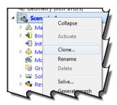
Clone Scenario 1 Change your Boundary Condition on Velocity from 12 to 60 mph Solve again from 0 to 100
