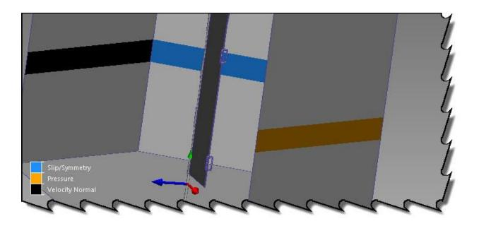
Model shown with Boundary Conditions applied as seen with the colored stripes on the surfaces.
