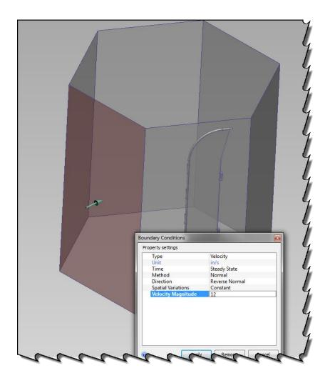
Apply the Slip/Symmetry to 4 of our 6 walls, this will allow the air to slide along the walls without changing any properties, speed and or force.
