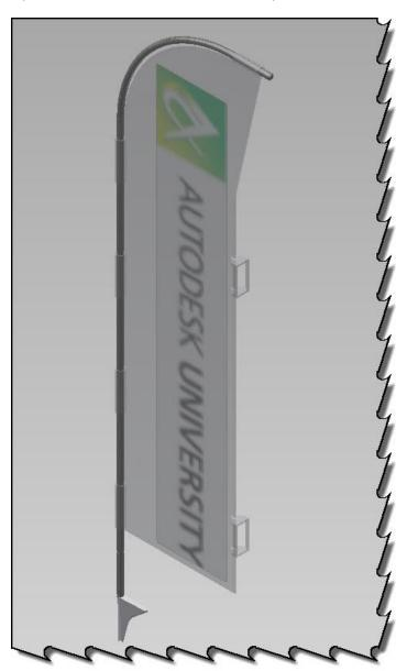
We need to create an environment for our wind to exist, or in our case turn that environment on; the visibility is turned off in our Inventor assembly file. Launch the model to Autodesk Simulation CFD
