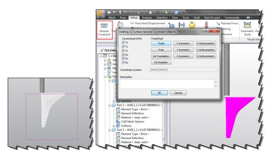
Window select the geometry as shown above, the surfaces to be held in place by solid material (Dirt, asphalt, Concrete etc.. ) and apply a General Constraint of *Fixed* and choose "OK" and fix them in place.
