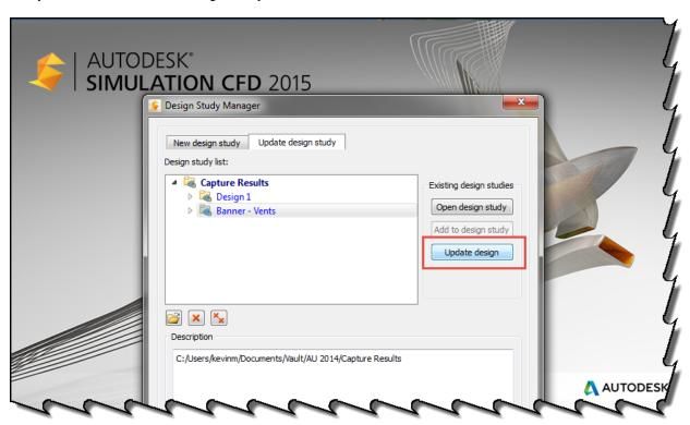
With the updated design in Simulation CFD you can perform another digital analysis with the new geometry in the model. Same steps as before using the Solve button be sure to continue from iteration 0 (zero).
