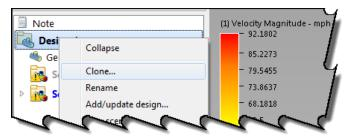
Now we need to bring the modified geometry into Simulation CFD. In Inventor 2015 activate the BANNER.ipt in the BANNER.iam file and move the End of Part down the bottom of the model tree. You will see 2 vents appear in the assembly. Follow the same steps as before only "Update design study" instead of the "New design study" as shown below.
