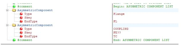
This type will be used by default only for flanges and couplings. Components which comply with the specific ISO Symbol Type, with the specific End Type and possibly with the specific SKEY will be recognized and presented accordingly in the isometric, which means that, for example, a flange will match its mating valve's isometric orientation.
