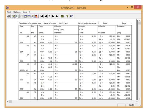
The results are also written to the pipes and sprinkler in the Revit model. They will be set in the shared parameters of pipes and sprinklers.
