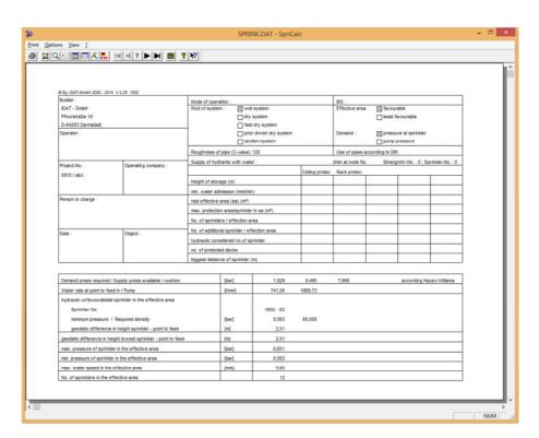
Some other forms show the results for pipes and sprinklers according to NFPA or VdS.
