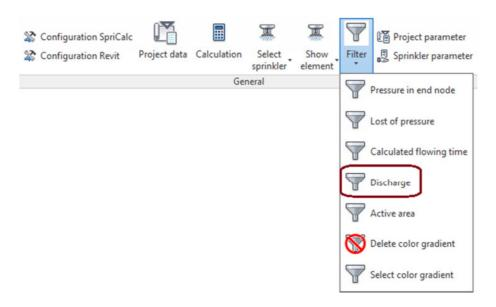
Now we can show different results of the calculation e.g. the discharge. In the configuration we had set colors to different levels of the discharge.
