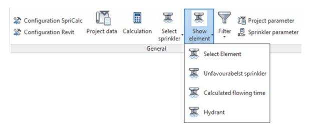
If we see the results in the calculation program it is easy to find the according element in the Revit model. We just need to enter the mark number and the program selects the pipe or the sprinkler for us.
