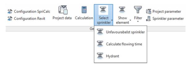
In the dialog of the previous chapter we can see the most unfavorable sprinkler at the mark 1604 and on the right side the sprinkler for flowing time calculation with the mark 1594. To set these mark numbers we can select sprinkler in Revit and then call the commands above.
