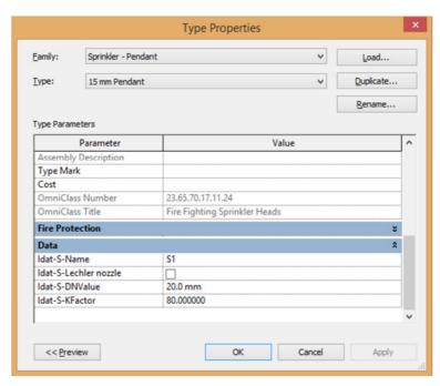
The data for the last four parameters of the pipes are set by the calculation program.
